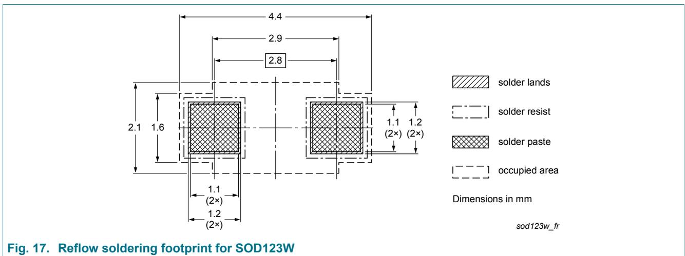
Fig. 17. Reflow soldering footprint for SOD123W
