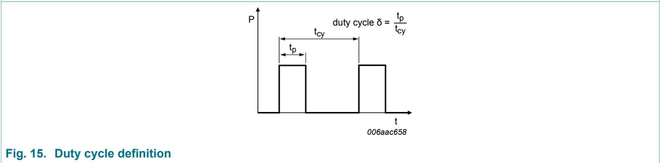
Fig. 15. Duty cycle definition
