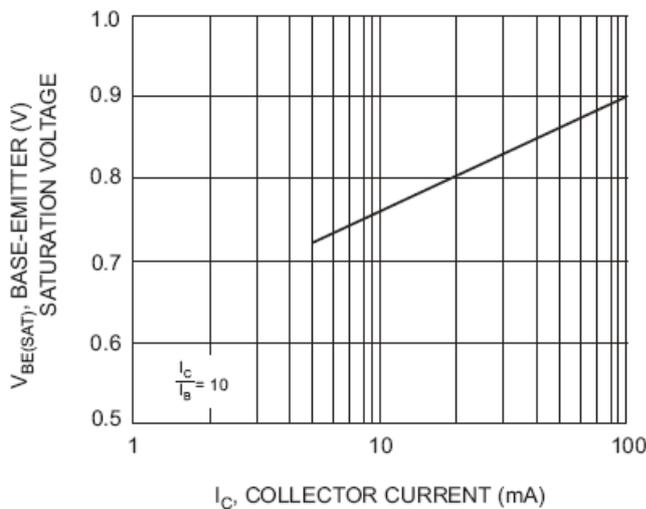
Fig. 5, Typical Base-Emitter Saturation Voltage vs. Collector Current
