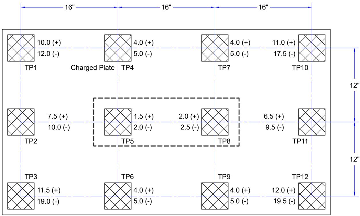
Figure 8. 50664 Neutralization (Discharge) Times at 120VAC, 60Hz input
