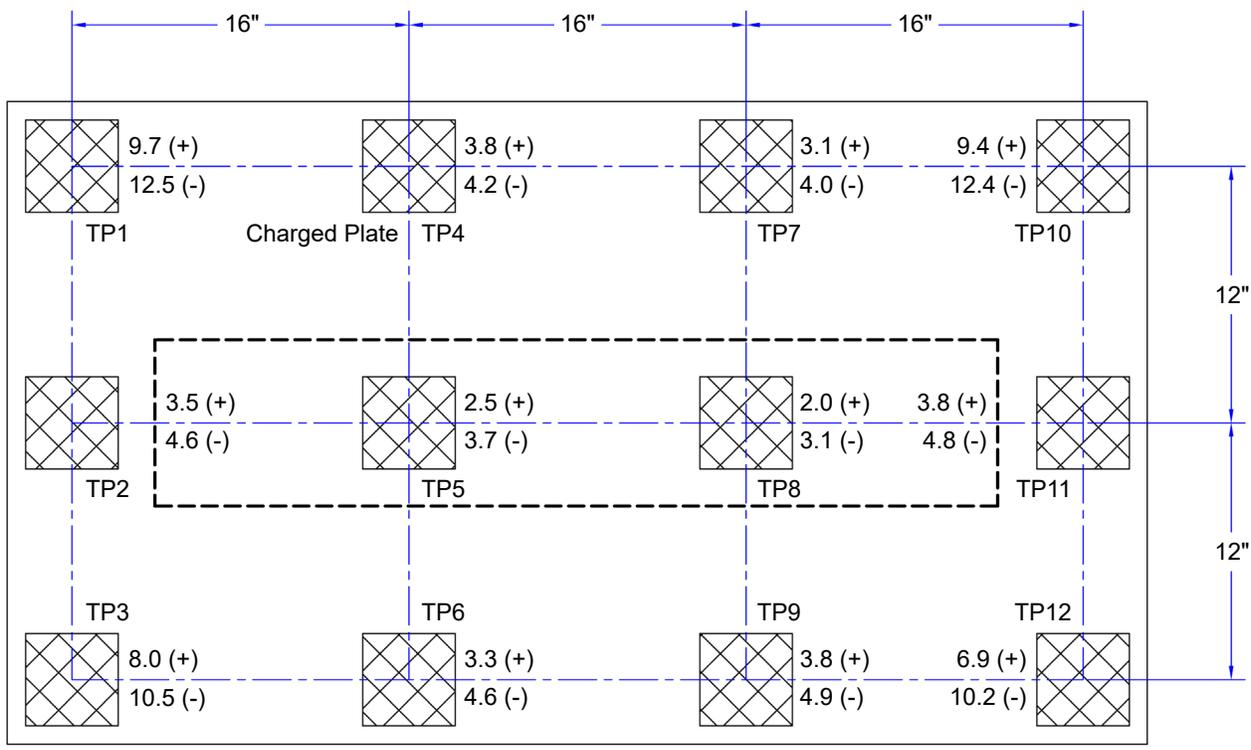
Figure 9. 50665 Neutralization (Discharge) Times at 100VAC, 50Hz input
