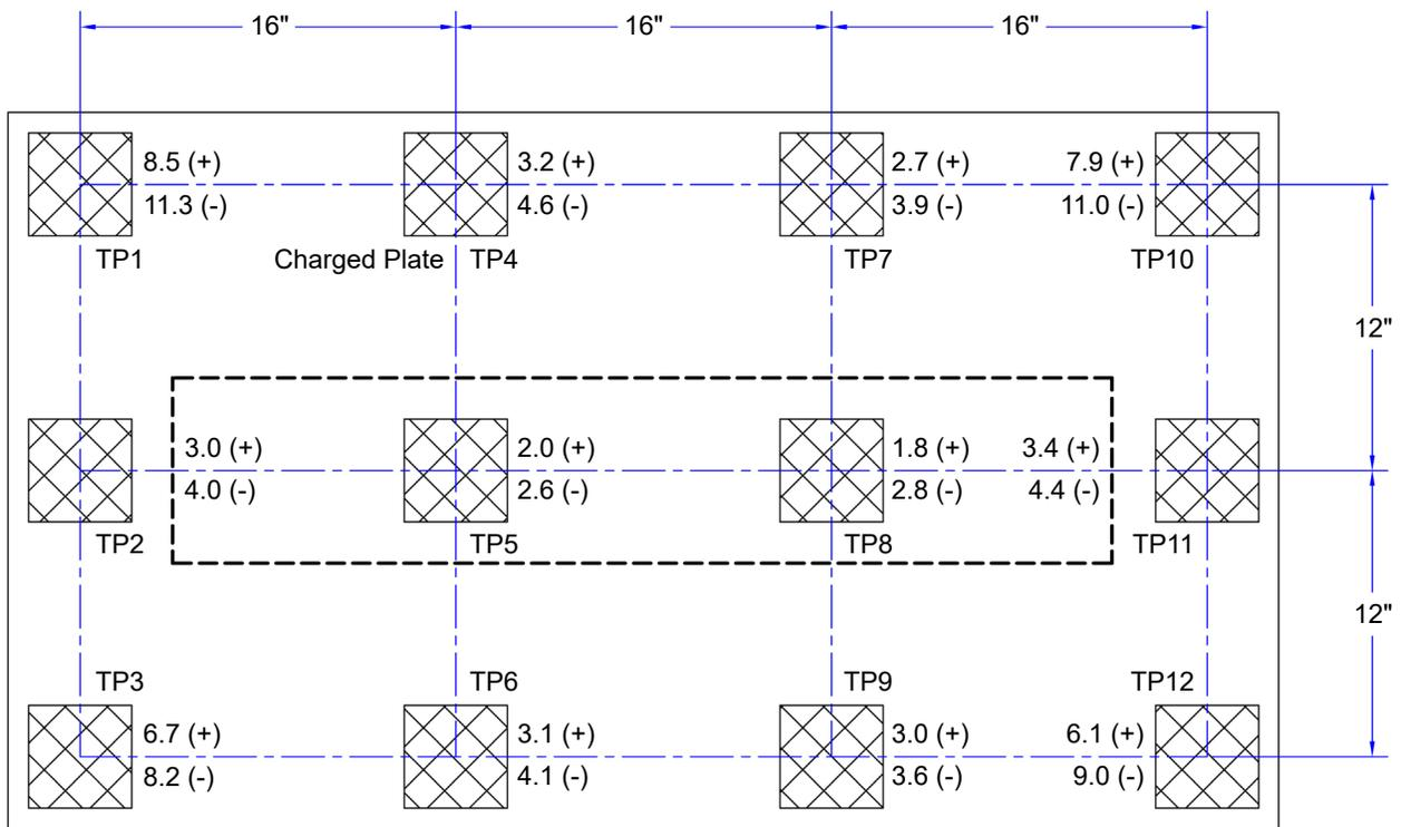
Figure 10. 50665 Neutralization (Discharge) Times at 120VAC, 60Hz input
