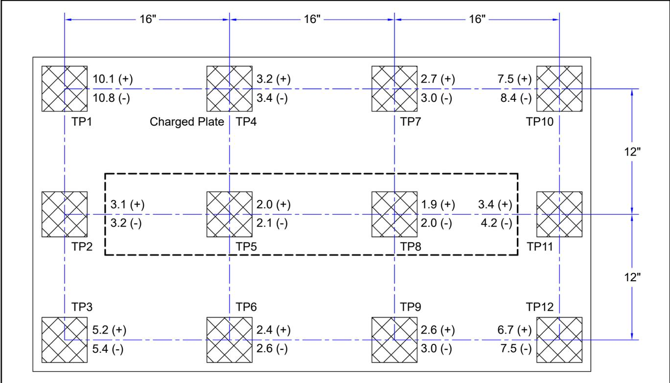
Figure 12. 50672 Neutralization (Discharge) Times at 220VAC, 50Hz input
