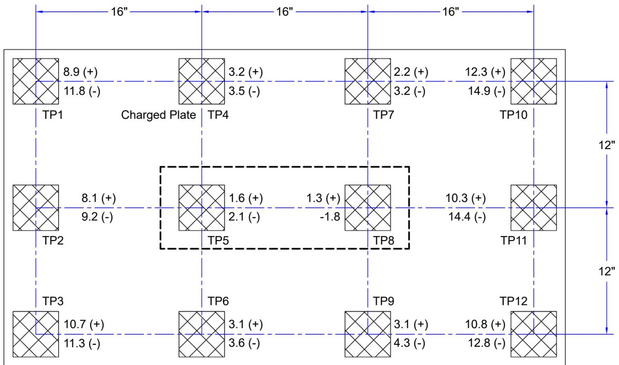
Figure 11. 50671 Neutralization (Discharge) Times at 220VAC, 50Hz input
