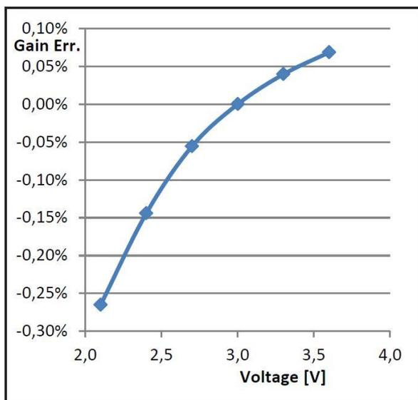
Data acquired like before with 100 pF ceramic COG capacitors connected “floating” in place of reference and sensor. The excitation capacitor was a 10 pF ceramics COG type.
