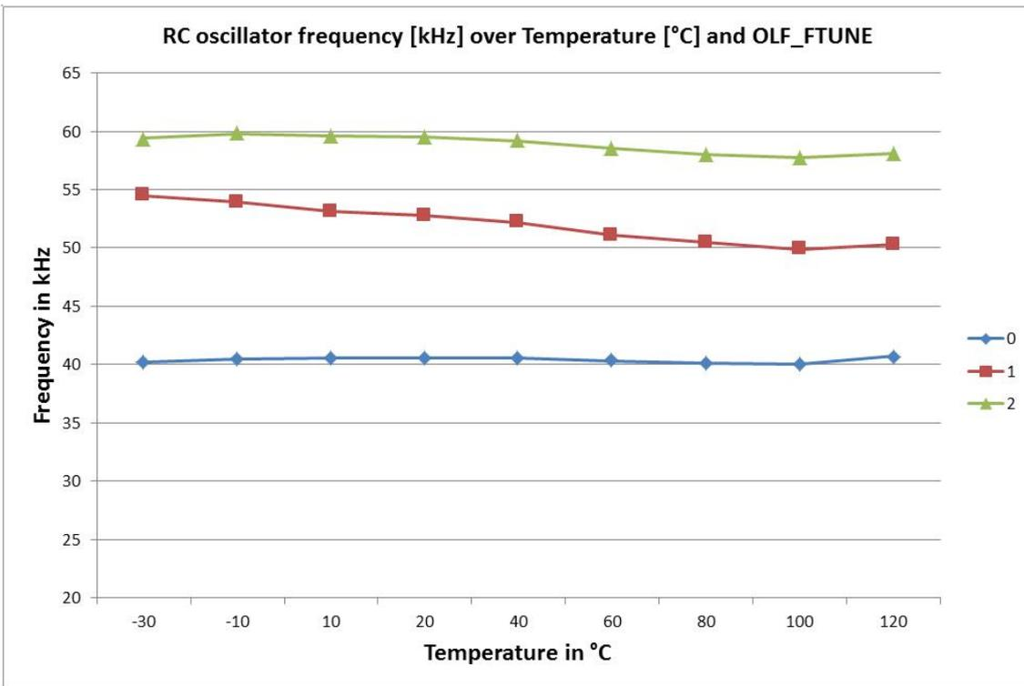
Figure 2-10: RC oscillator frequency dependence on temperature and OLF\_FTUNE setting 0-2
