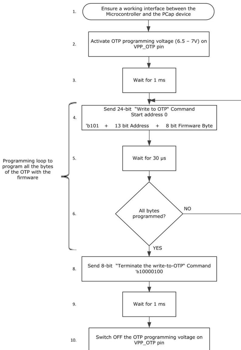
sequence of steps to be performed to program the firmware into the OTP:
