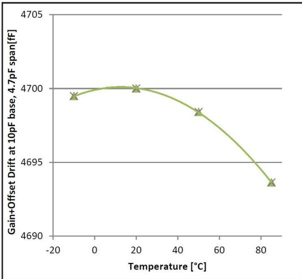
Gain drift as a function of temperature at 3.0V supply voltage VDD. 10 pF base capacitance, both sensor and reference, plus 4.7 pF span, with COG ceramics capacitors each, connected “floating”.
