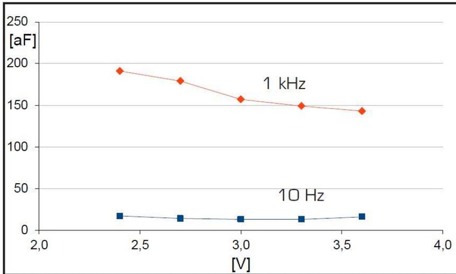
Figure 2-4 RMS Noise vs. Supply Voltage
