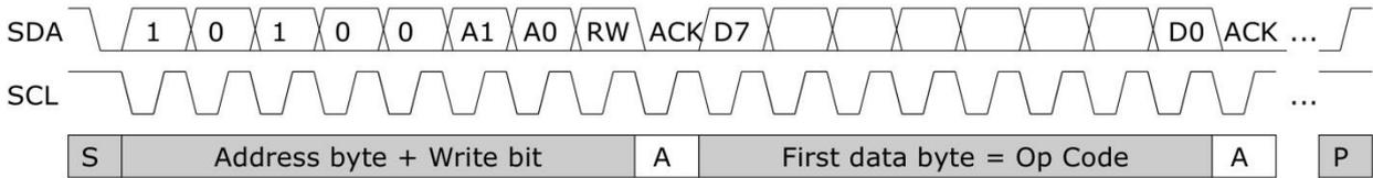
Figure 4-1: I<sup>2</sup>C principle sequence
