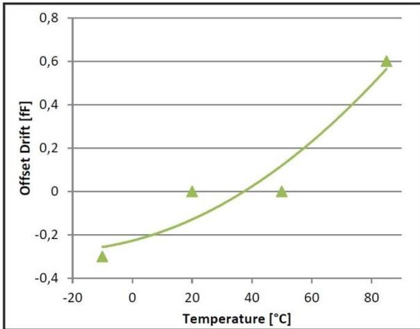
Offset drift as a function of temperature at 3.0V supply voltage VDD. 10 pF base capacitance, both sensor and reference, a COG ceramics capacitor each, connected “floating”.
