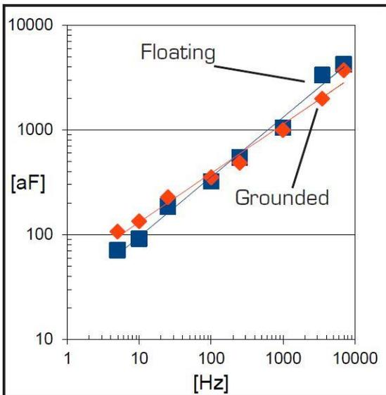
Figure 2-3 Typical Capacitive Noise vs. Output Data Rate, with 100 pF Base Capacitance, V = 3.0 V
