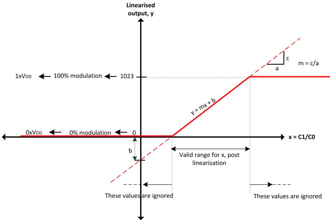
Figure 4-8: PWM-PDM linearization
