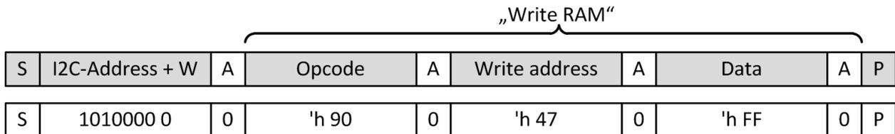
Figure 4-2 I<sup>2</sup>C Write, an example
