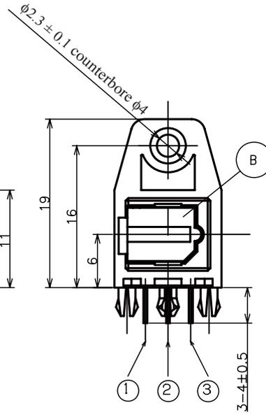
Example of mounting drawing from solder side.
