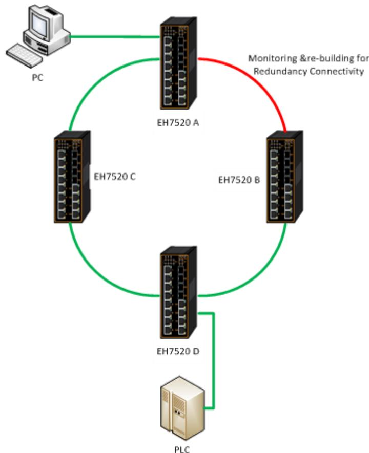
Figure 2.151 iA-Ring Example Topology (Example made on EH7520)
