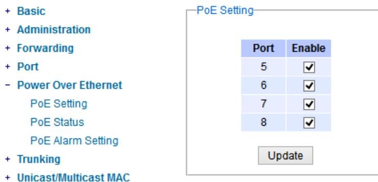
Figure 2.73 Power over Ethernet Dropdown Menu example on EHG7508-4SFP-4PoE
