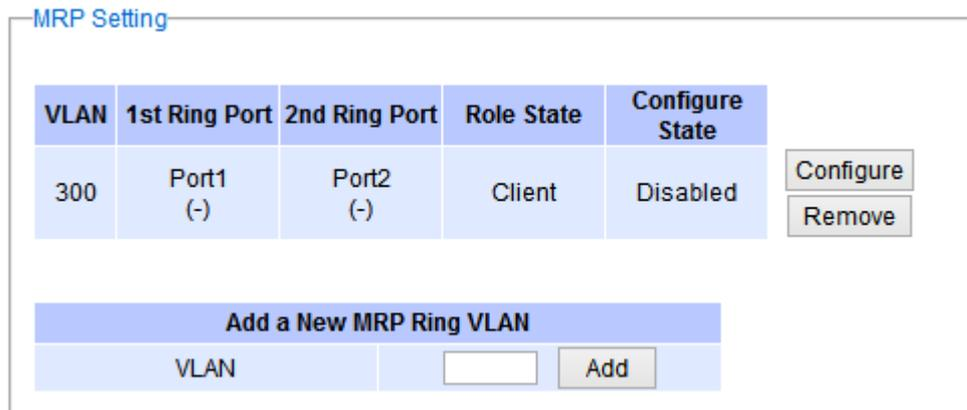
Figure 2.166 Example of PROFINET's MRP VLAN Entry
