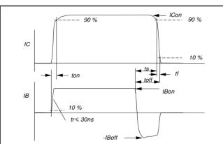
Fig.4. Switching times waveforms with resistive load.
