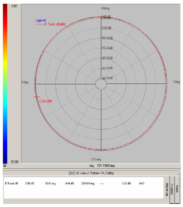
Frequency (MHz): 2450.00 Pattern Field: H Plane Average Gain: 0.22dB
