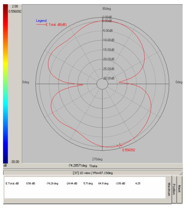
Frequency (MHz): 2450.00 Pattern Field: E Plane Average Gain: -3.5 dB
