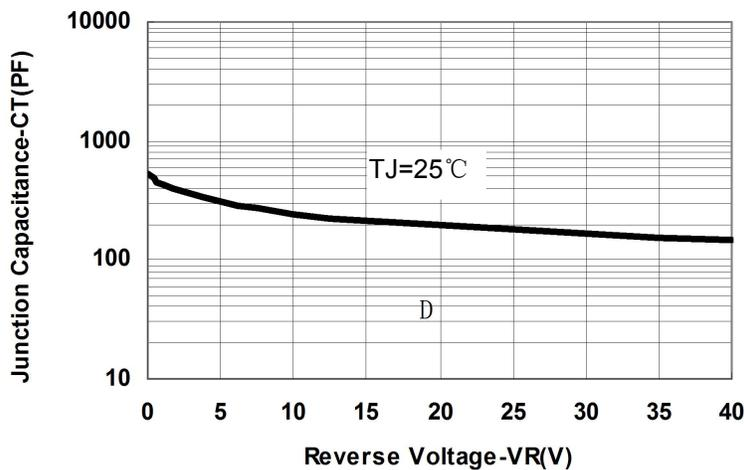
Fig.1-Typical Junction Capacitance
