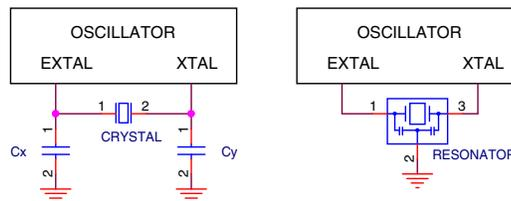
**Figure 37. Crystal connection – Diagram 2**
