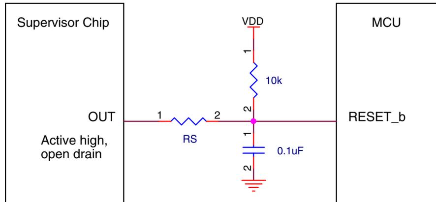
**Figure 33. Reset signal connection to external reset chip**
