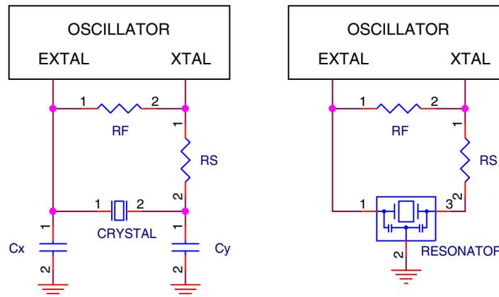
**Figure 38. Crystal connection – Diagram 3****NOTE**
