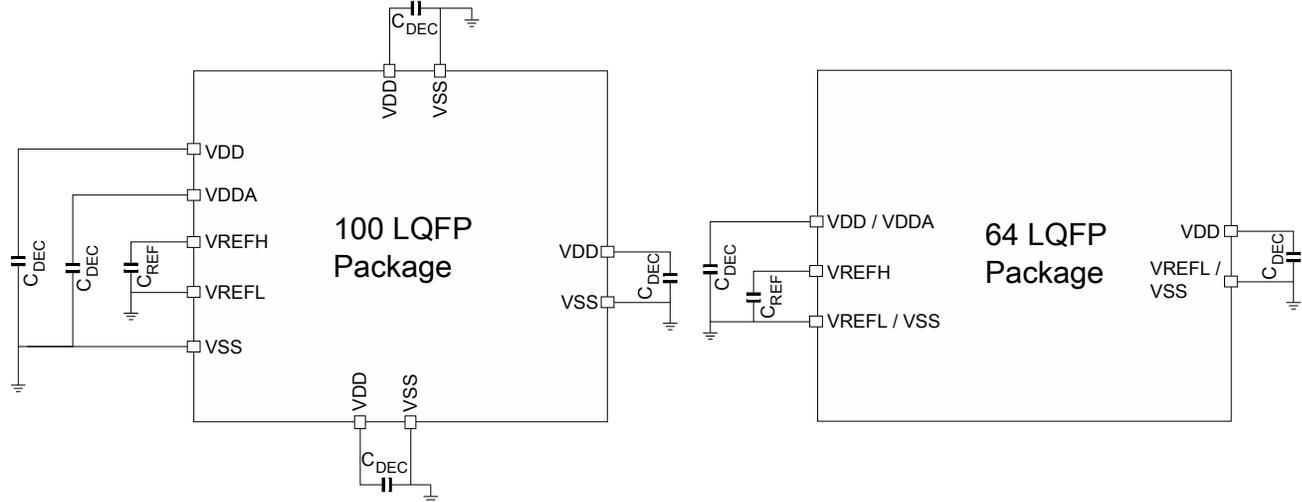
Figure 13. Pinout decoupling
