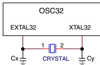
Figure 36. RTC Oscillator (OSC32) module connection – Diagram 1
