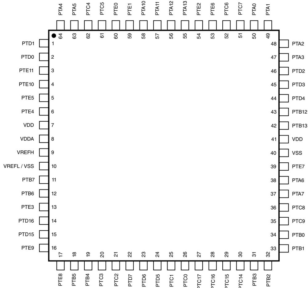
Figure 8. 64 LQFP Pinout Diagram
