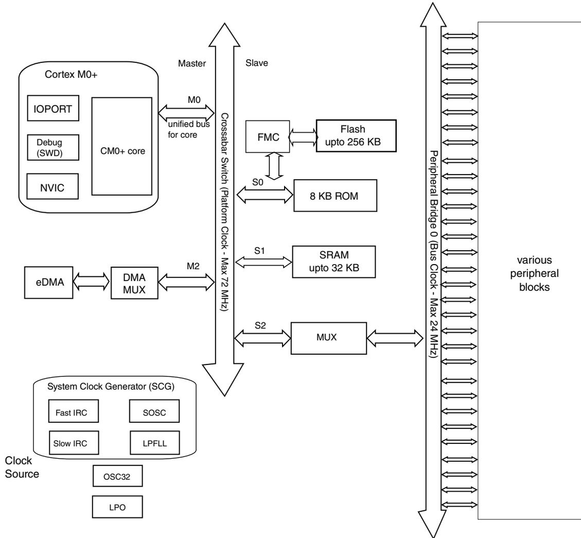
**Figure 2. System diagram**
