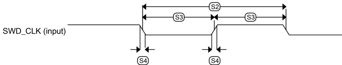
**Figure 28. Serial wire clock input timing**
