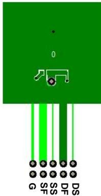
a. 38  $^{\circ}\text{C}/\text{W}$  when mounted on a 1 in<sup>2</sup> pad of 2 oz copper
