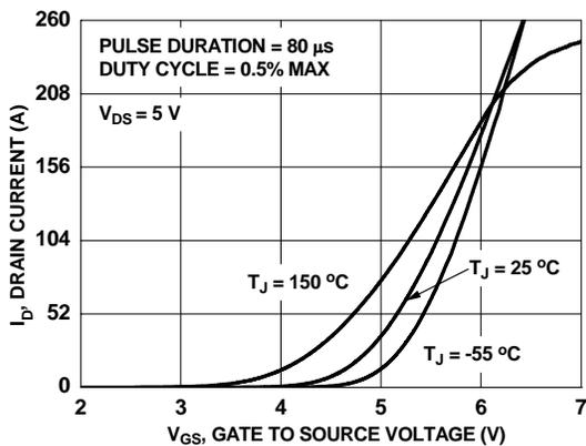
**Figure 5. Transfer Characteristics**
