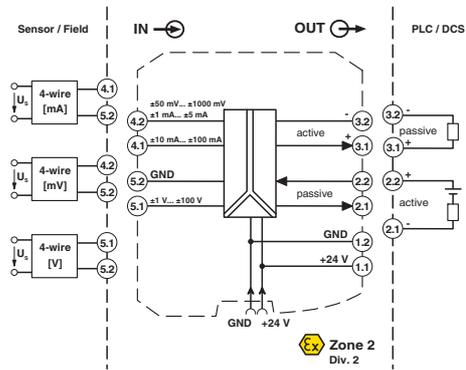
Figure 1 Block diagram with connection terminal blocks
