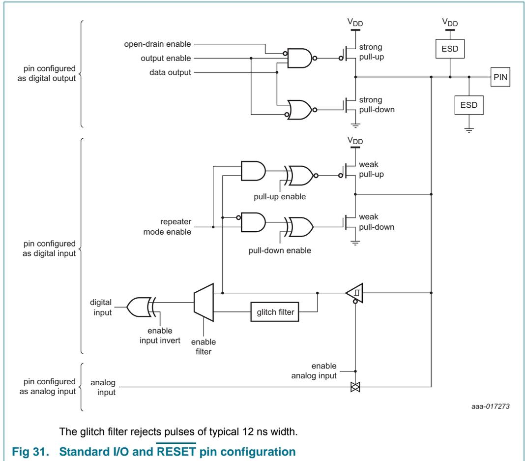
**Fig 31. Standard I/O and RESET pin configuration**
