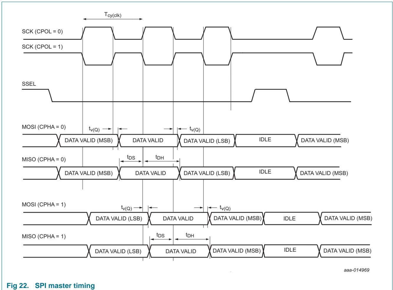
**Fig 22. SPI master timing**
