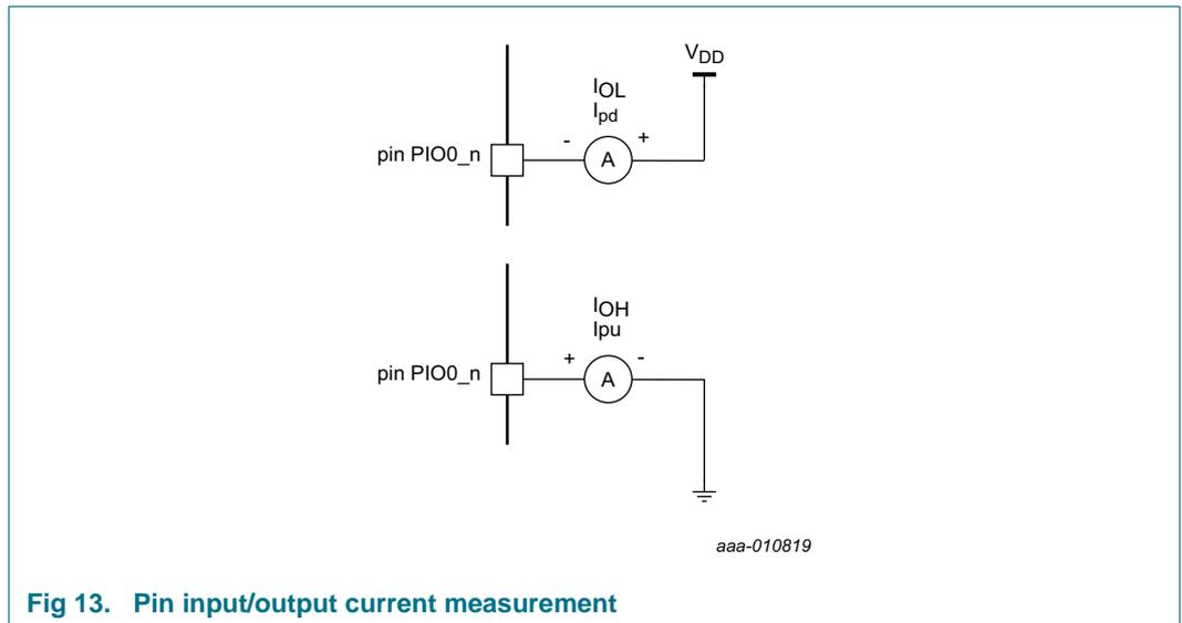
**Fig 13. Pin input/output current measurement**
