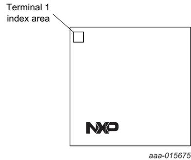
Fig 2. WLCSP49 package marking
