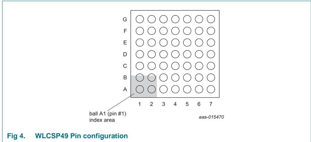
Fig 4. WLCSP49 Pin configuration
