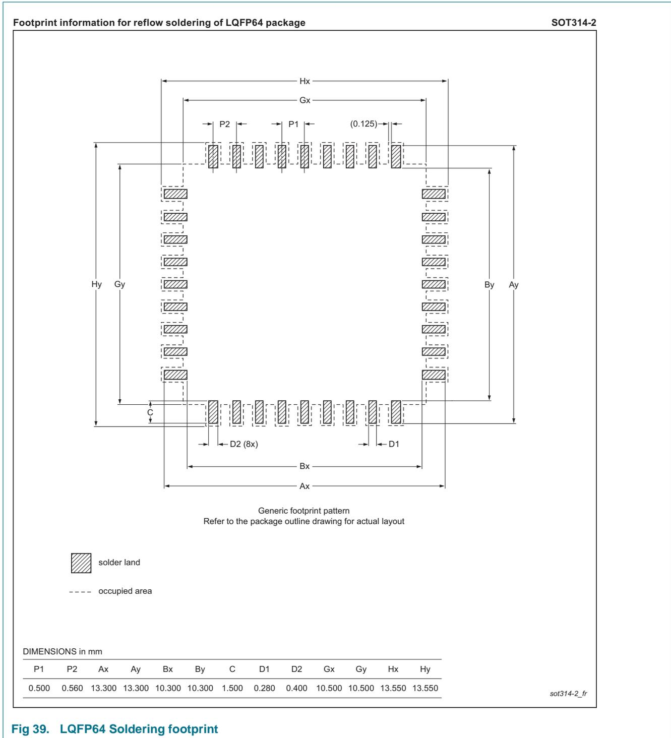
Fig 39. LQFP64 Soldering footprint
