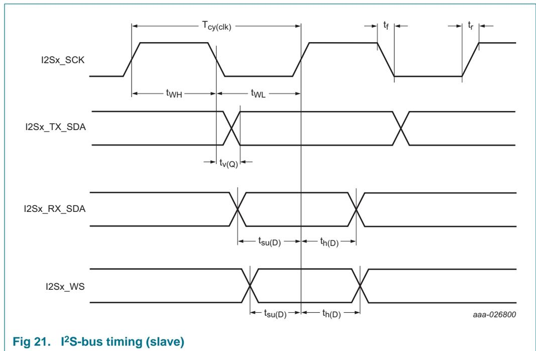
Fig 21. I<sup>2</sup>S-bus timing (slave)
