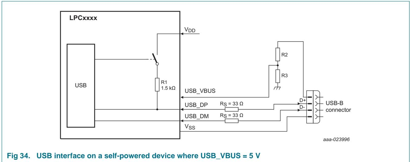
**Fig 34. USB interface on a self-powered device where USB\_VBUS = 5 V**
