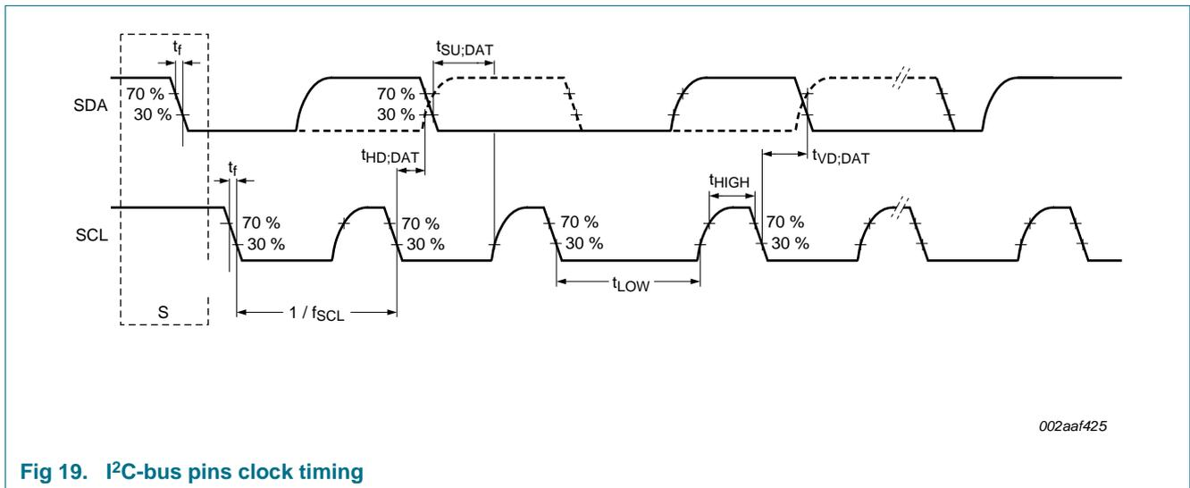
Fig 19. I<sup>2</sup>C-bus pins clock timing
