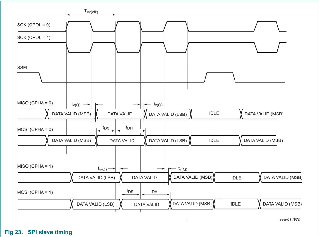
Fig 23. SPI slave timing
