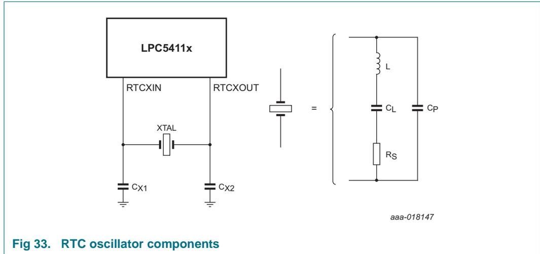
**Fig 33. RTC oscillator components**
