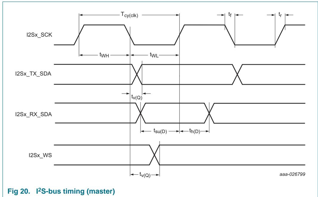
Fig 20. I<sup>2</sup>S-bus timing (master)
