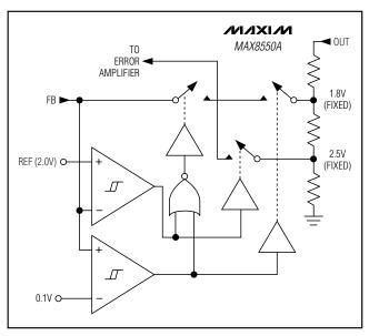
Figure 5. Dual-Mode Feedback Decoder
