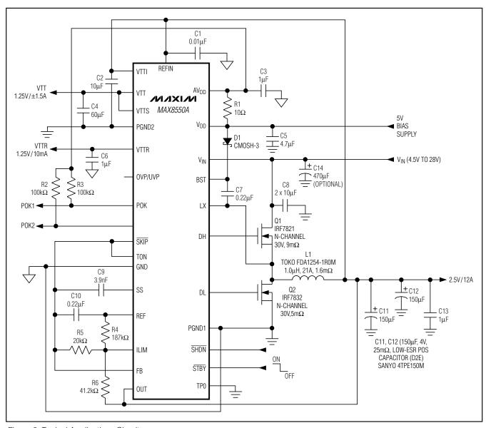
Figure 8. Typical Applications Circuit
