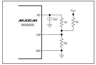
Figure 7. Foldback Current Limit
