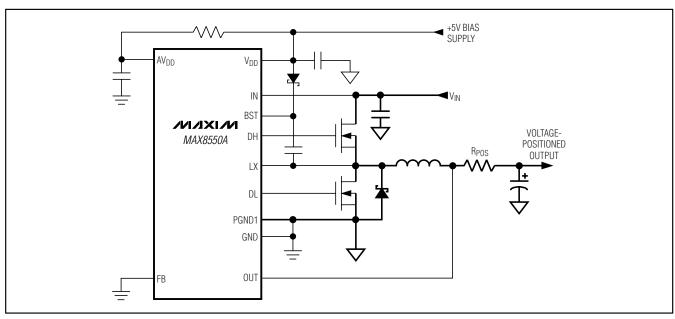
Figure 9. Voltage-Positioned Output
