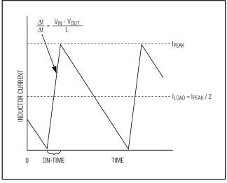
Figure 2. Pulse-Skipping/Discontinuous Crossover Point
