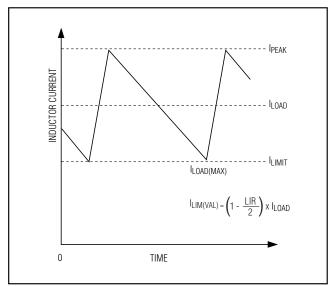
Figure 4. Valley Current-Limit Threshold
