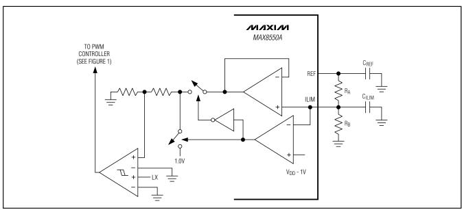
Figure 3. Adjustable Current-Limit Threshold
