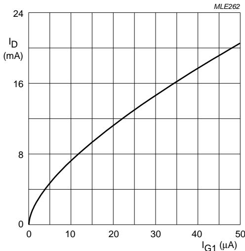
$V_{DS} = 5$  V;  $V_{G2-S} = 4$  V;  $T_j = 25$  °C.
