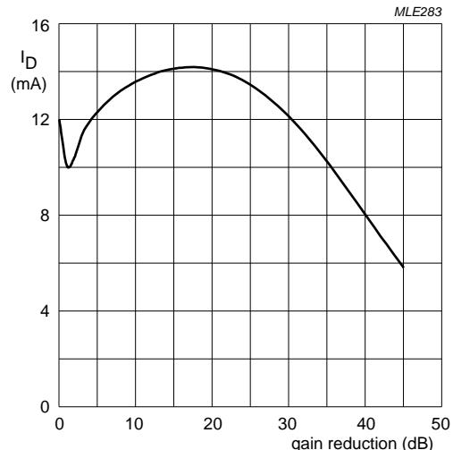
$V_{DS} = 5$  V;  $V_{GG} = 5$  V;  $R_{G1} = 150$  kΩ;  $f = 50$  MHz;  $T_{amb} = 25$  °C;
