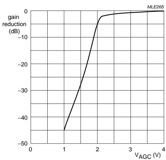
$V_{DS} = 5$  V;  $V_{GG} = 5$  V;  $R_{G1} = 91$  kΩ;  $f = 50$  MHz;  $T_{amb} = 25$  °C;
