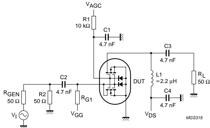
Fig.35 Cross-modulation test set-up (for one MOS-FET).
