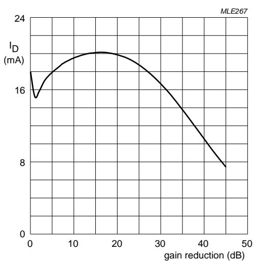
$V_{DS} = 5$  V;  $V_{GG} = 5$  V;  $R_{G1} = 91$  kΩ;  $f = 50$  MHz;  $T_{amb} = 25$  °C;
