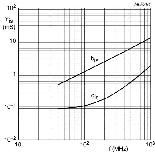
$V_{DS} = 5$  V;  $V_{G2} = 4$  V;  $I_D = 12$  mA;  $T_{amb} = 25$  °C.
