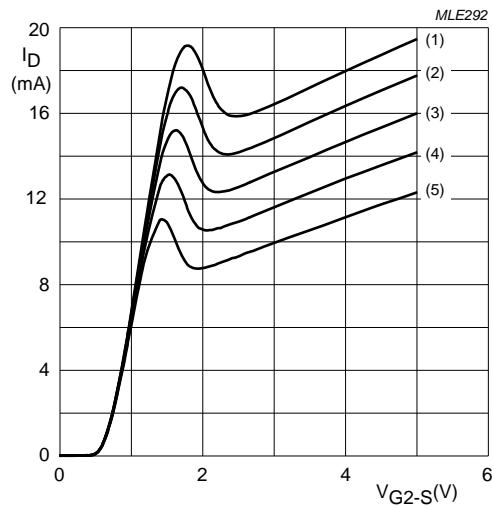
$V_{DS} = 5$  V;  $T_j = 25$  °C;  $R_{G1} = 91$  kΩ (connected to  $V_{GG}$ ); see Fig.35.
