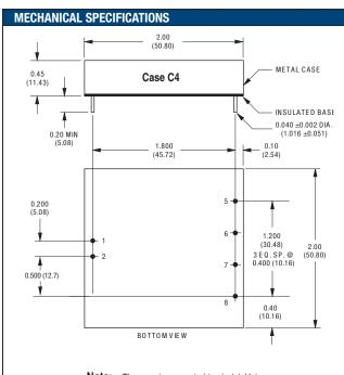
**Note:** The case is connected to pin 1 (+V<sub>IN</sub>).
