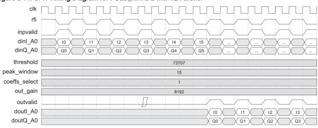
Figure 2-11. CFR Timing Diagram for FOLD\_RATE 2 with IQ Parallel
