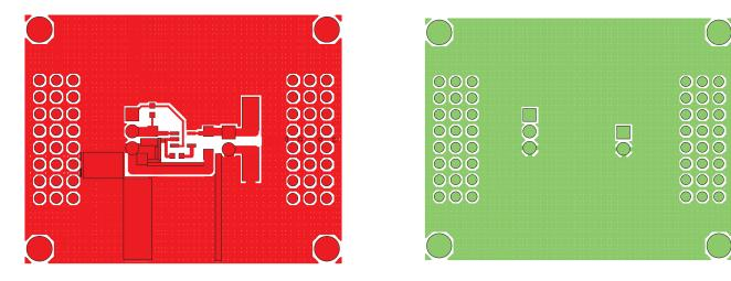
Figure 3: Evaluation Board Component Side Layout.
