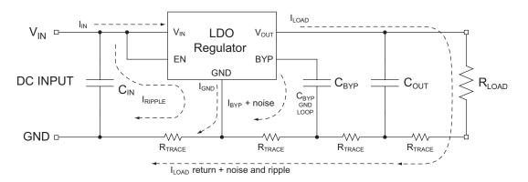
Figure 1: Common LDO Regulator Layout with C<sub>BYP</sub> Ripple Feedback Loop.
