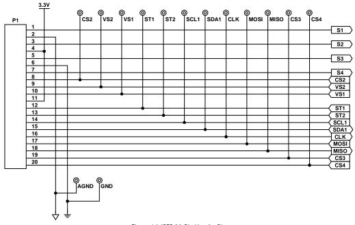
Figure 16. ISEB 20-Pin Header Pinout
