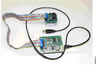
Figure 1. Inertial Sensor Evaluation System
