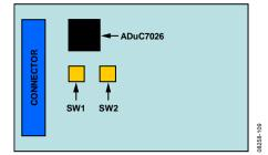
Figure 9. ISEB Switch Locations for Flashing the Microcontroller
