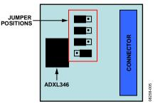
Figure 5. Correct Jumper Positions for the ADXL346 Satellite
