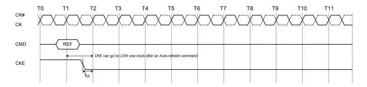
Figure 56. Active command to power-down entry
