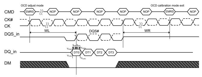
NOTE 1: For proper operation of adjust mode, WL = RL - 1 = AL + CL - 1t<sub>CK</sub> and t<sub>DS</sub>/t<sub>DH</sub> should be met as shown in the figure. NOTE 2: For input data pattern for adjustment, DT0-DT3 is a fixed order and is not affected by burst type (i.e., sequential or interleave)
