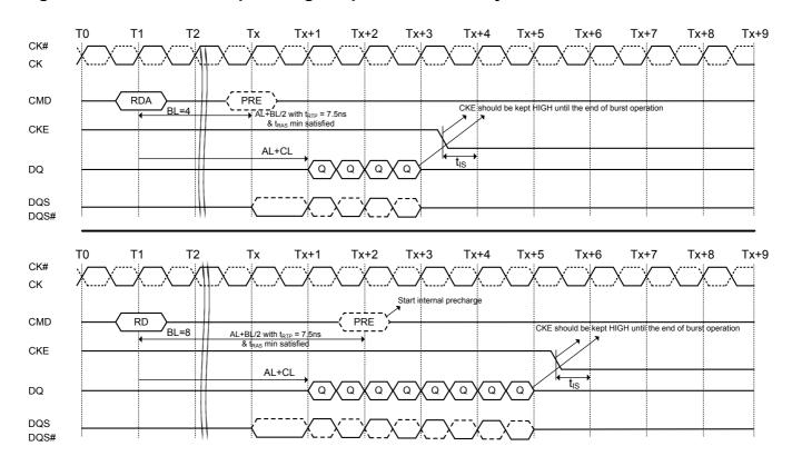
Figure 53. Write to power-down entry
