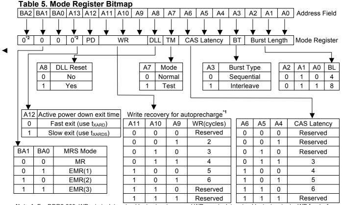
Note 1: For DDR2-800, WR min is determined by  $t_{CK}$  (avg) max and WR max is determined by  $t_{CK}$ (avg) min. WR [cycles] = RU { $t_{WR}$ [ns]/ $t_{CK}$ (avg)[ns]}, where RU stands for round up. The mode register must be programmed to this value. This is also used with  $t_{RP}$  to determine  $t_{DAL}$ .
