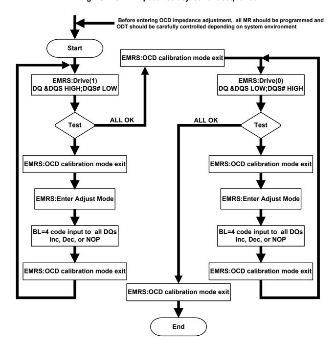
Figure 4. OCD impedance adjustment sequence
