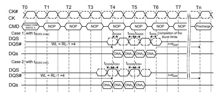
Figure 28. Burst write operation: RL=3 (AL=0, CL=3), WL=2, BL=4
