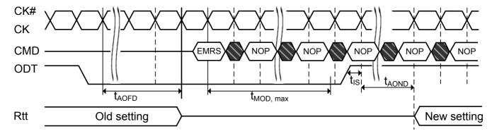
NOTE 1: EMRS command directed to EMR(1), which updates the information in EMR(1)[A6,A2], i.e. Rtt (Nominal). NOTE 2: "setting" in this diagram is measured from outside.
