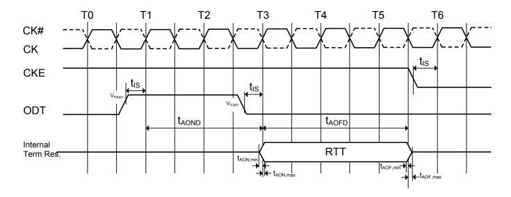
Figure 14. ODT timing for power-down mode
