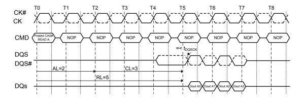
Figure 22. Burst read operation: RL=3 (AL=0, CL=3, BL=8)
