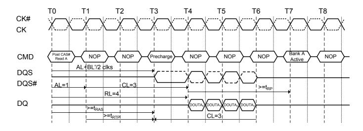
Figure 34. Burst read operation followed by precharge: (RL=4, AL=1, CL=3, BL=8, t<sub>RTP</sub>≤2 clocks)
