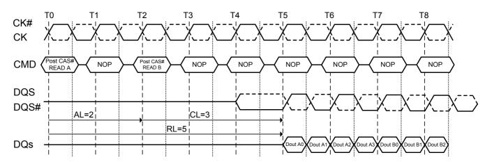
NOTE: The seamless burst read operation is supported by enabling a read command at every other clock for BL = 4 operation, and every 4 clock for BL = 8 operation. This operation is allowed regardless of same or different banks as long as the banks are activated.
