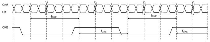
NOTE: DRAM guarantees all AC and DC timing & voltage specifications and proper DLL operation with intensive CKE operation
