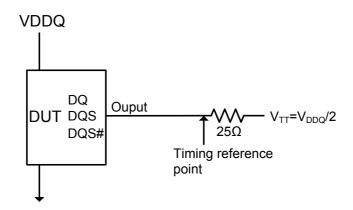
The output timing reference voltage level for single ended signals is the crosspoint with VTT. The output timing reference voltage level for differential signals is the crosspoint of the true (e.g. DQS) and the complement (e.g. DQS#) signal.
