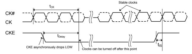
Figure 60. Clock frequency change in precharge power down mode
