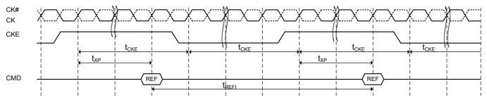
NOTE: The pattern shown above can repeat over a long period of time. With this pattern, DRAM guarantees all AC and DC timing & voltage specifications and DLL operation with temperature and voltage drift
