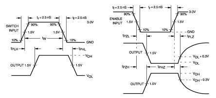
FIGURE 2. AC Waveforms
