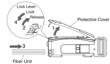
When mounting a coaxial reflective Fiber Unit, insert the single-core Fiber unit to the upper hole (Emitter side) and the multi-core Fiber Unit to the lower hole (Receiver side).
