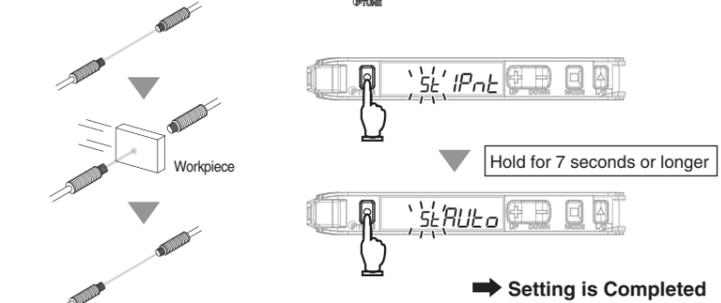
Incident light level setting: Adjust the max. incident light level on Step 1 as the power tuning level.
