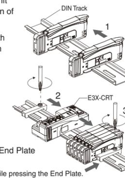
Up to 30 Amplifier Units can be connected to E3X-ECT Communication Unit.
