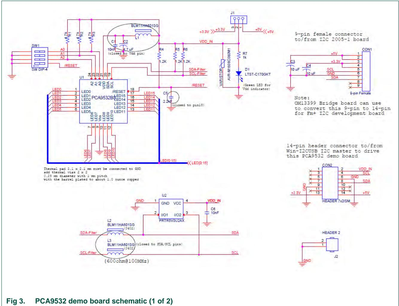
Fig 3. PCA9532 demo board schematic (1 of 2)
