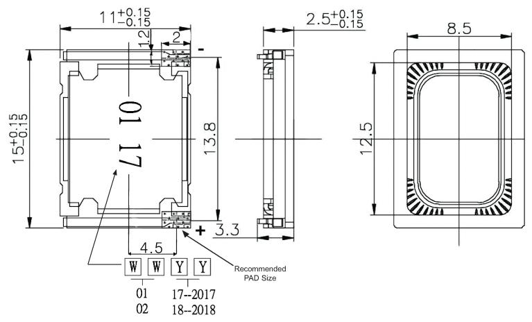
1. Maximum compression force between front frame and back frame & yoke is 5 N.
