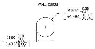
\*UNLESS OTHERWISE SPECIFIED TOLERANCES PER DECIMAL PRECISION ARE: X=±1 (±0.039), X.X=±0.5 (±0.020), X.XX=±0.25 (±0.010), X.XXX=±0.127 (±0.005). LEAD SIZE=±0.05 (±0.002), LEAD LENGTH=±0.75 (±0.030). MIN= +DECIMAL PRECISION MAX. = +0.00 -DECIMAL PRECISION
