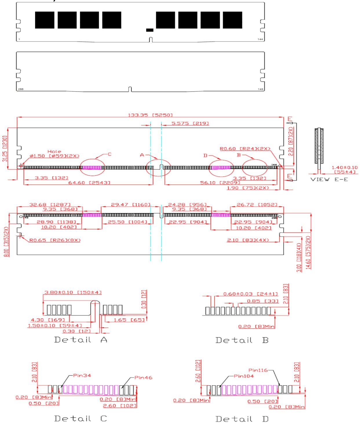
Note: All dimensions are in millimeters(mils) and should be kept within a tolerance of  $\pm 0.15(5.91)$ ,unless otherwise specified..
