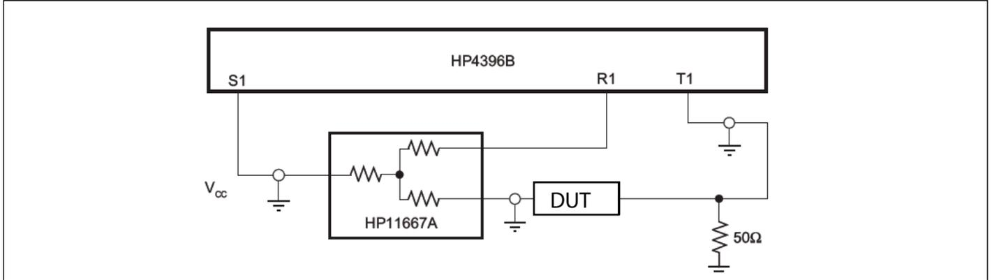
**Test Circuit for Electrical Characteristics**
