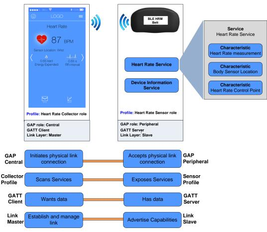
The Heart Rate Profile contains a Heart Rate Service and a Device Information Service. Within the Heart Rate Service, there are three Characteristics, each containing different information. The device in the diagram is configured as a Sensor role, meaning that in the context of the Heart Rate Profile, the device is a GAP Peripheral and a GATT Server. These concepts are explained in the BLE Stack description.
