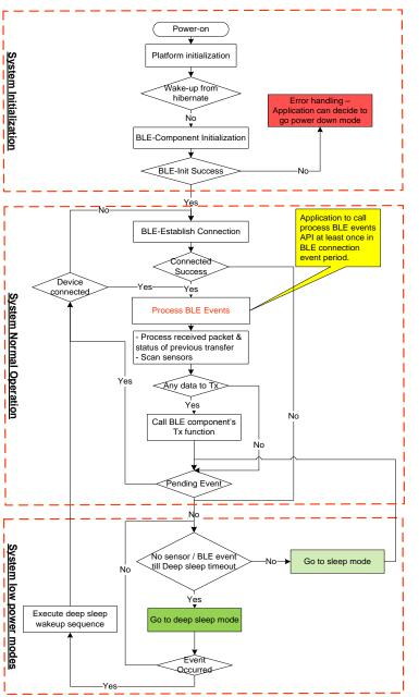
Once the Component is initialized, it enters normal operation and periodically enters various degrees of low power operation to conserve power. Hence initialization should only happen at
