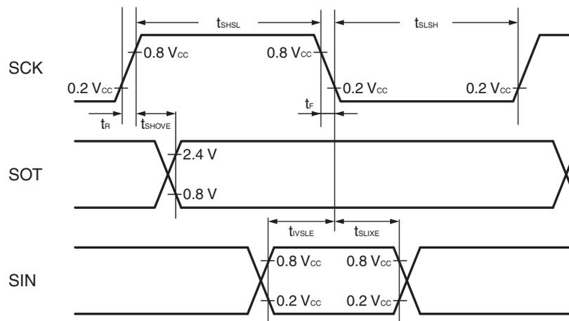
Sampling is executed at the rising edge of the sampling clock\*1, and serial clock delay is enabled\*2. (ESCR register : SCES bit = 0, ECCR register : SCDE bit = 1)
