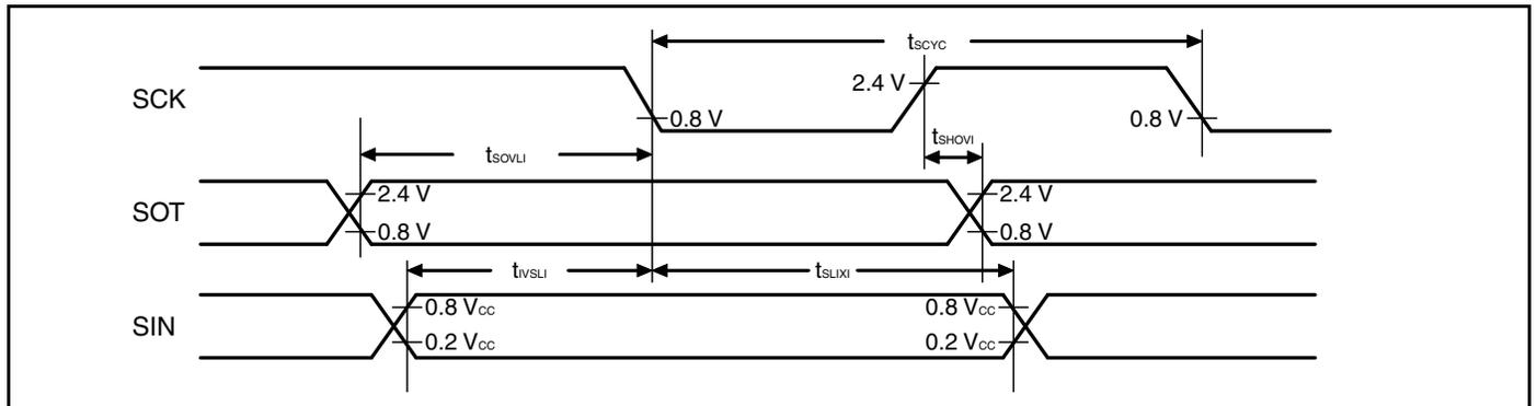
Sampling is executed at the falling edge of the sampling clock\*1, and serial clock delay is enabled\*2.
