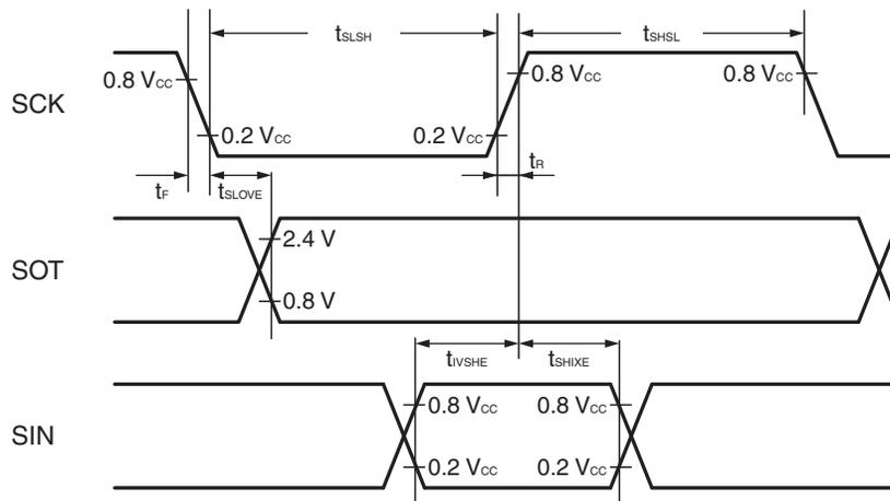
Sampling is executed at the falling edge of the sampling clock\*1, and serial clock delay is disabled\*2. (ESCR register : SCES bit = 1, ECCR register : SCDE bit = 0)
