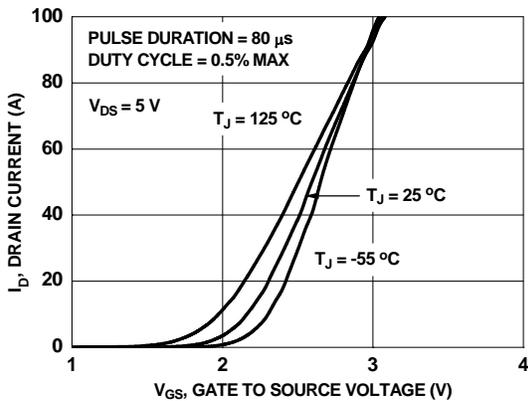
**Figure 5. Transfer Characteristics**
