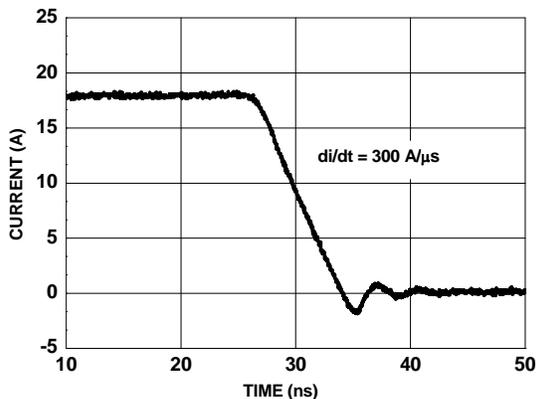
Figure 14. FDMS0312AS SyncFET body diode reverse recovery characteristic
