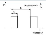
Fig. 14. Duty cycle definition
