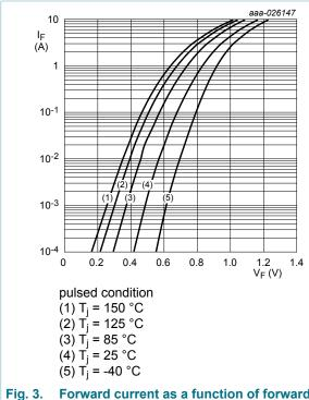
ig. 3. Forward current as a function of forward voltage; typical values
