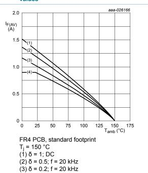
Fig. 8. Average forward current as a function of ambient temperature; typical values
