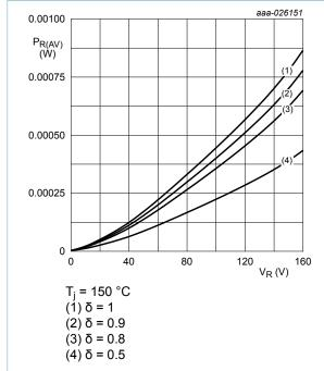
Fig. 7. Average reverse power dissipation as a function of reverse voltage; typical values
