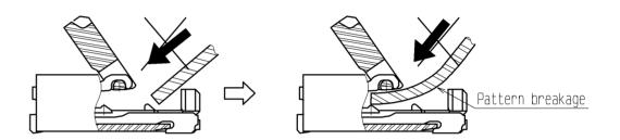
3. Do not rotate the actuator when FPC TAB is on Metal Fittings.
