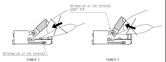
2. The actuator rotates around the rotational axis as shown below. Rotate the actuator.
