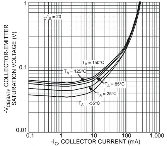
Fig. 7 Typical Collector-Emitter Saturation Voltage vs. Collector Current
