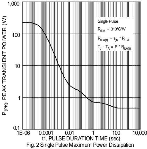
Fig. 2 Single Pulse Maximum Power Dissipation
