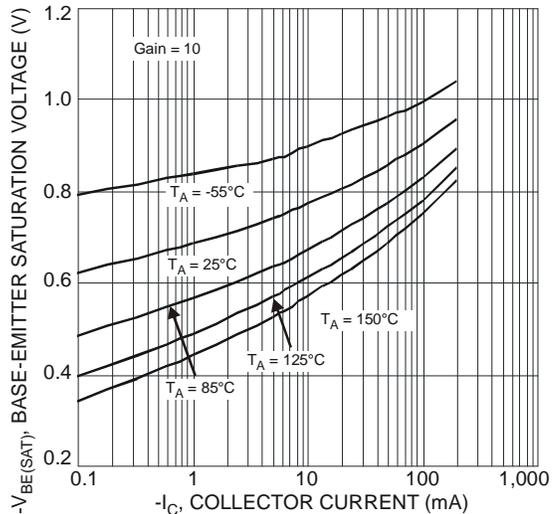
Fig. 9 Typical Base-Emitter Saturation Voltage vs. Collector Current
