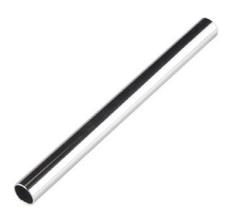
**Description:** These 8" long aluminum tubes have an outer diameter of  $\frac{1}{2}$ ", an inner diameter of 0.444", and a wall thickness of 0.03". When used with the mating tube clamps, these can be used for versatile structural support. Additionally, wires and cables can easily be run through the center.
