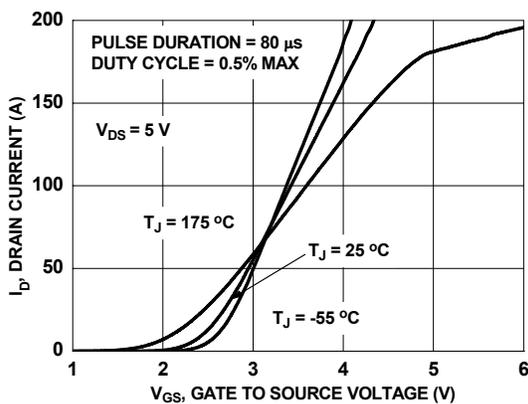
**Figure 5. Transfer Characteristics**
