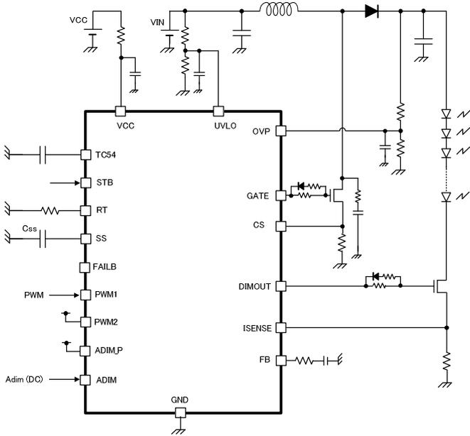
Figure 17. the circuit example with single PWM (1)
