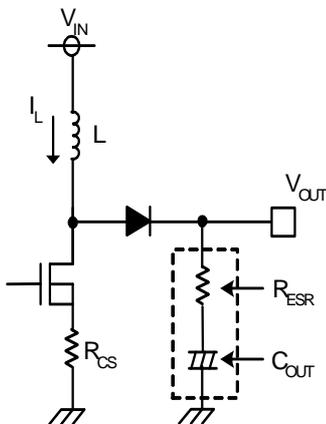
Output capacitor needs to be selected in consideration of equivalent series resistance required to even the stable area of output voltage or ripple voltage. Be aware that set LED current may not be flown due to decrease in LED terminal voltage if output ripple component is high.
