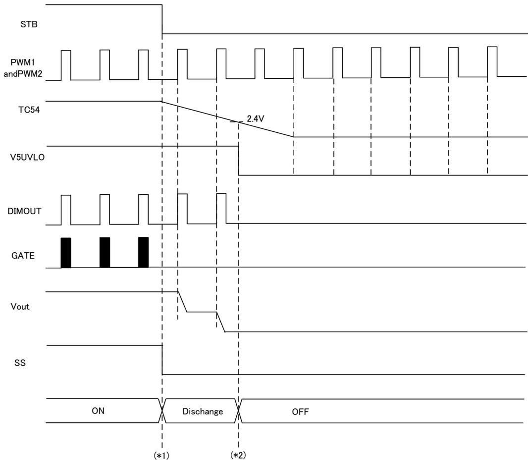
(\*1)...As STB pin turns High to Low, BD9285F stops the boost operation, starts the discharge of TC54.
