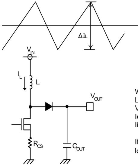
The inductor value affects the input ripple current. The equality in the section 3.5.1 is as following.
