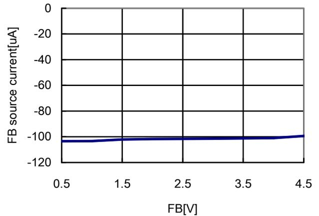
Figure 9. FB source current vs FB voltage
