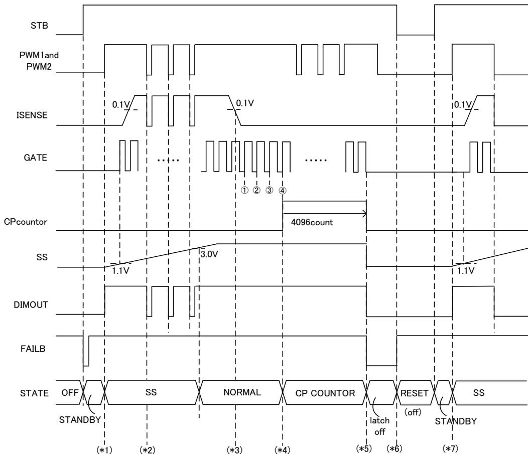
(\*1)...During starting up, even if the normality,  $I_{SENSE} < 0.1V$  because of the low  $V_{out}$ . Therefore the OPEN detection will be masked for the soft start period.
