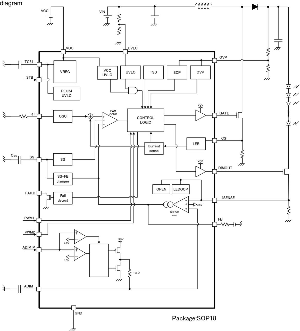
Figure 5. Block diagram
