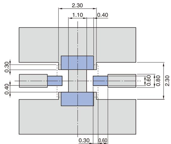
Line width should be designed to match 50Ω characteristic impedance, depending on PCB material and thickness.
