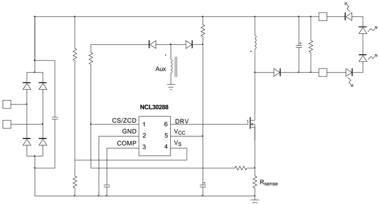
Figure 2. Typical Application Schematic in a Buck-Boost Converter
