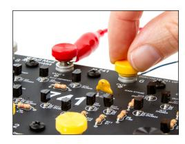
You can connect to the 741 through bare wire, alligator clips, or spade or ring lugs, using the terminal posts. You can also directly solder wires to the small pins next to each terminal post, if you're careful to clip the wires such that they don't touch the aluminum legs.
