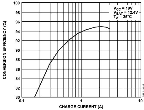
Figure 15. Conversion Efficiency vs. Charge Current
