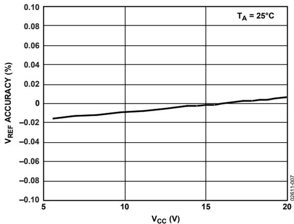
Figure 7.  $V_{REF}$  Accuracy vs.  $V_{CC}$
