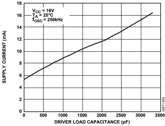
Figure 9. Supply Current vs. Driver Load Capacitance
