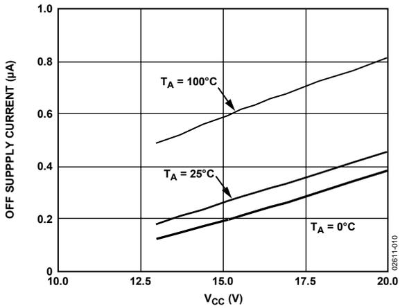
Figure 10. Off Supply Current vs.  $V_{CC}$
