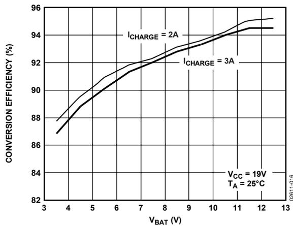
Figure 16. Conversion Efficiency vs. Battery Voltage
