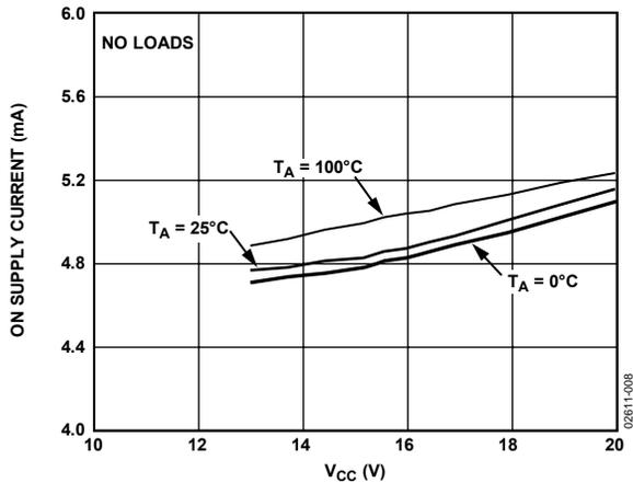
Figure 8. On Supply Current vs.  $V_{CC}$
