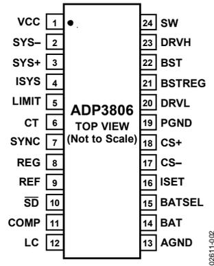
Figure 2. Pin Configuration
