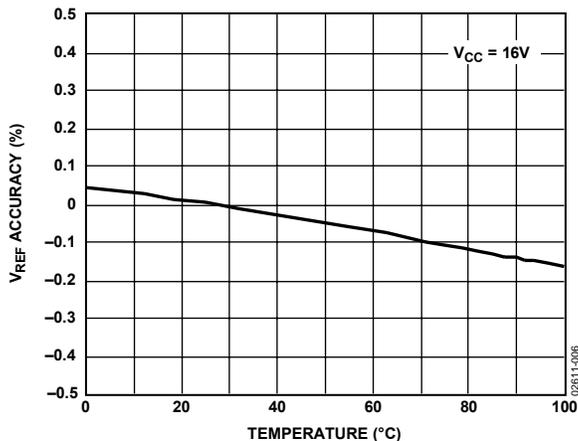
Figure 6.  $V_{REF}$  Accuracy vs. Temperature
