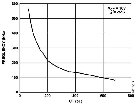
Figure 11. Oscillator Frequency vs.  $CT$
