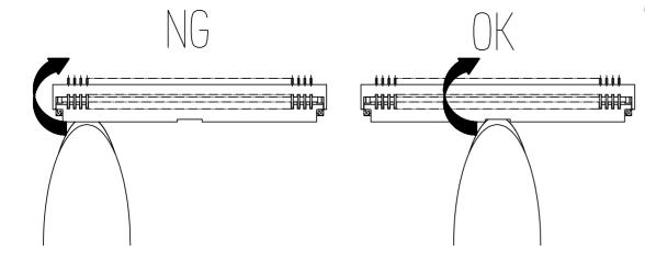
5. Do not lift or snag the actuator as shown in the figures below. This can result in damage. (Operate the actuator only in a rotating fashion as instructed in paragraph 2 above.)
