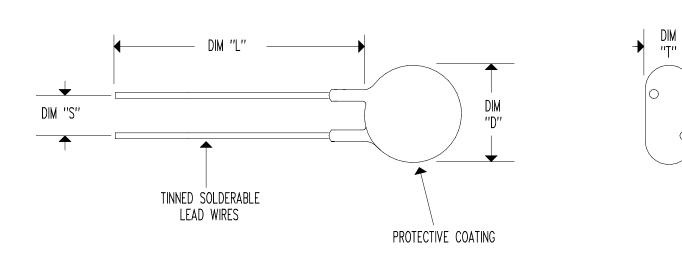
RESISTANCE @  $+25^{\circ}C=30~\Omega~\pm~20\%$  MAXIMUM STEADY STATE CURRENT = 3 AMPS RESISTANCE @ MAXIMUM CURRENT = 0.46  $\Omega$  NOMINAL
