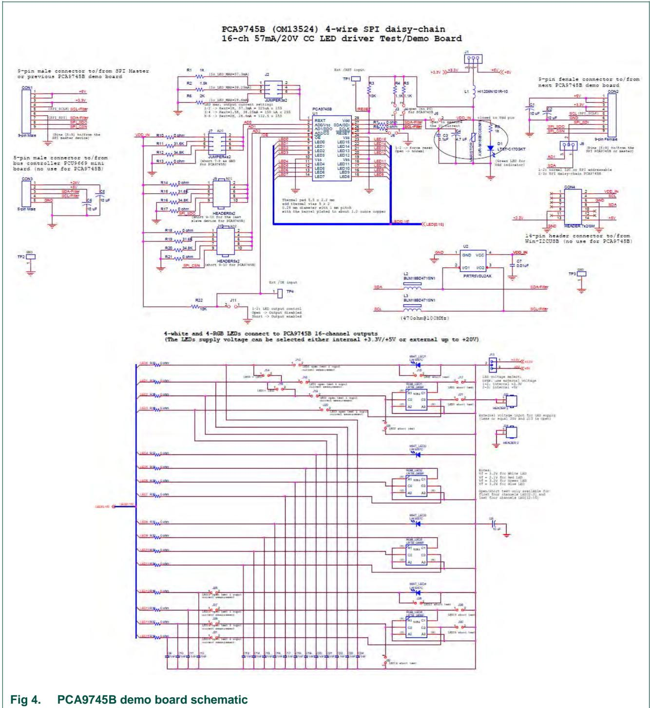
Fig 4. PCA9745B demo board schematic
