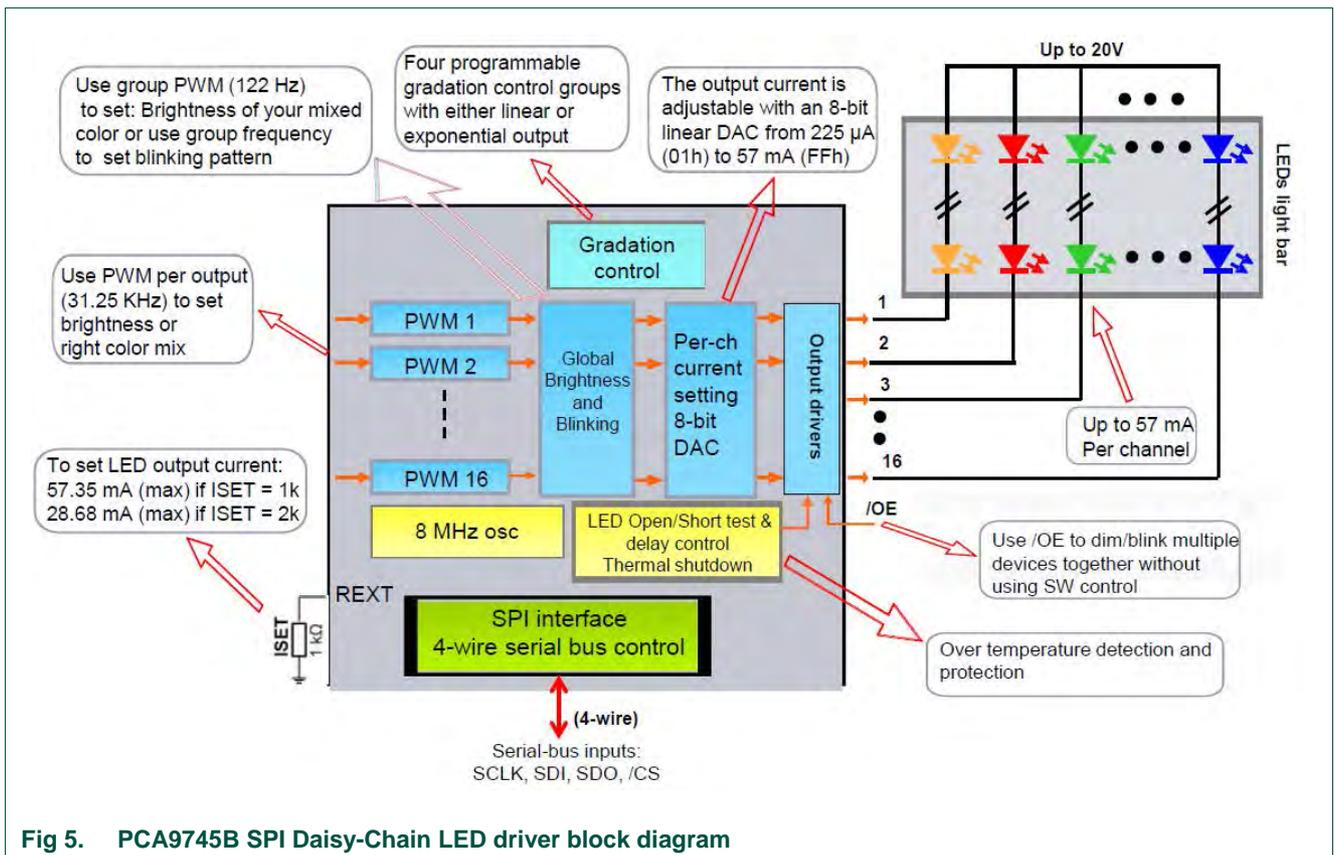
**Fig 5. PCA9745B SPI Daisy-Chain LED driver block diagram**
