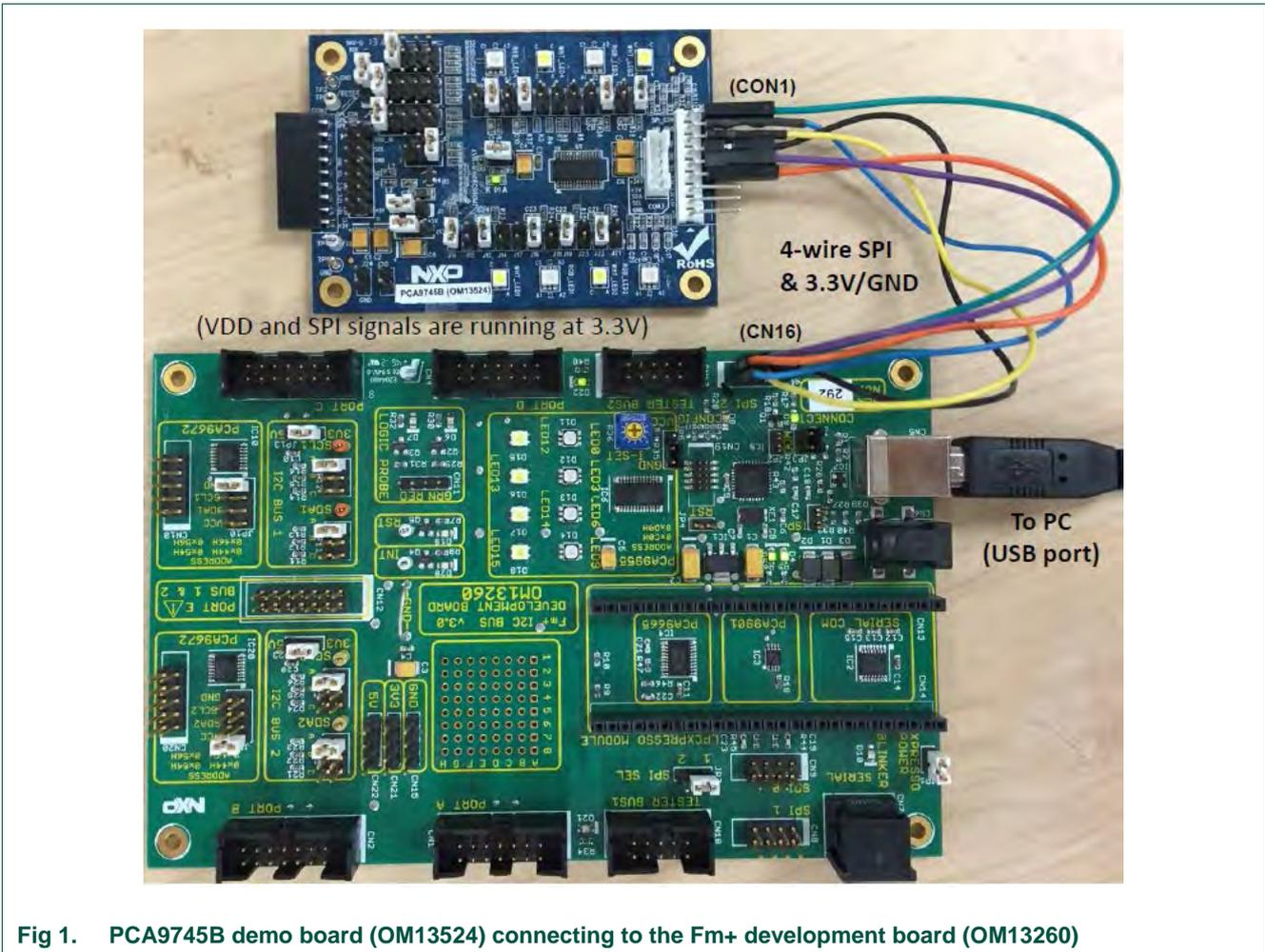
Fig 1. PCA9745B demo board (OM13524) connecting to the Fm+ development board (OM13260)
