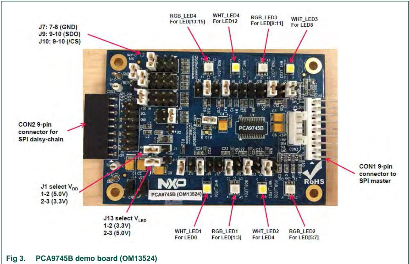
Fig 3. PCA9745B demo board (OM13524)
