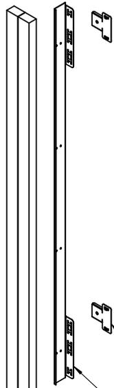
MOUNTING BRACKETS ATTACHED TO RAILS
