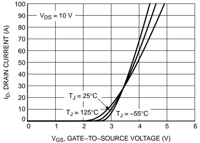
Figure 2. Transfer Characteristics
