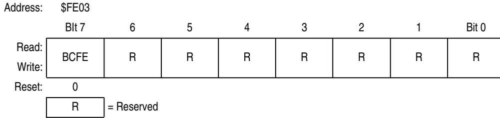
**Figure 14-16. SIM Break Flag Control Register (SBFCR)**
