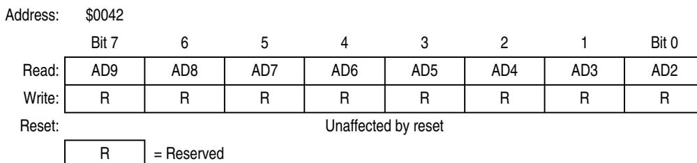
**Figure 3-9. ADC Data Register Low (ADRL) 8-Bit Mode**
