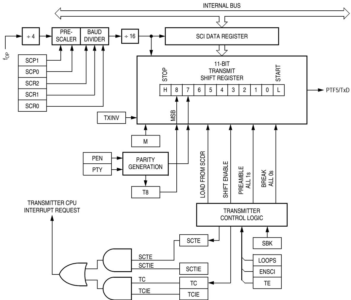
Figure 13-5. SCI Transmitter
