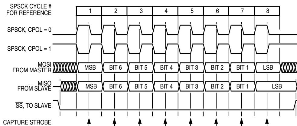
Figure 15-7. Transmission Format ( $CPHA = 1$ )
