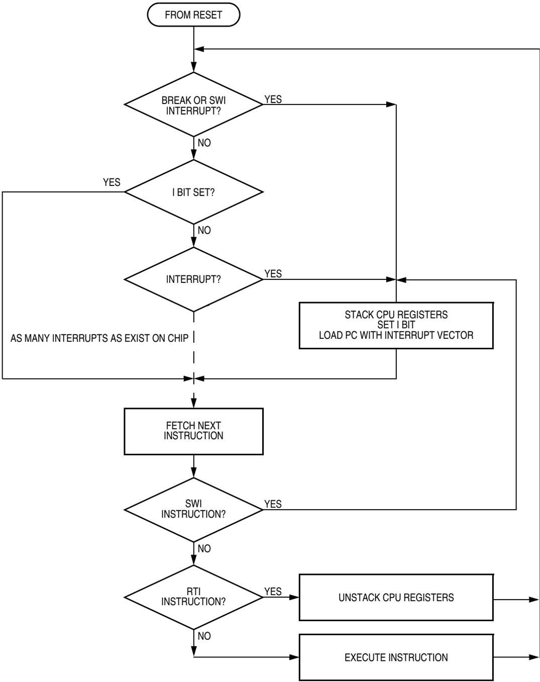
Figure 14-8. Interrupt Processing
