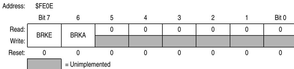
**Figure 18-3. Break Status and Control Register (BRKSCR)**
