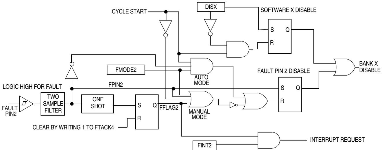
The example is of fault pin 2 with DISX. Fault pin 4 with DISY is logically similar and affects BANK Y disable.
