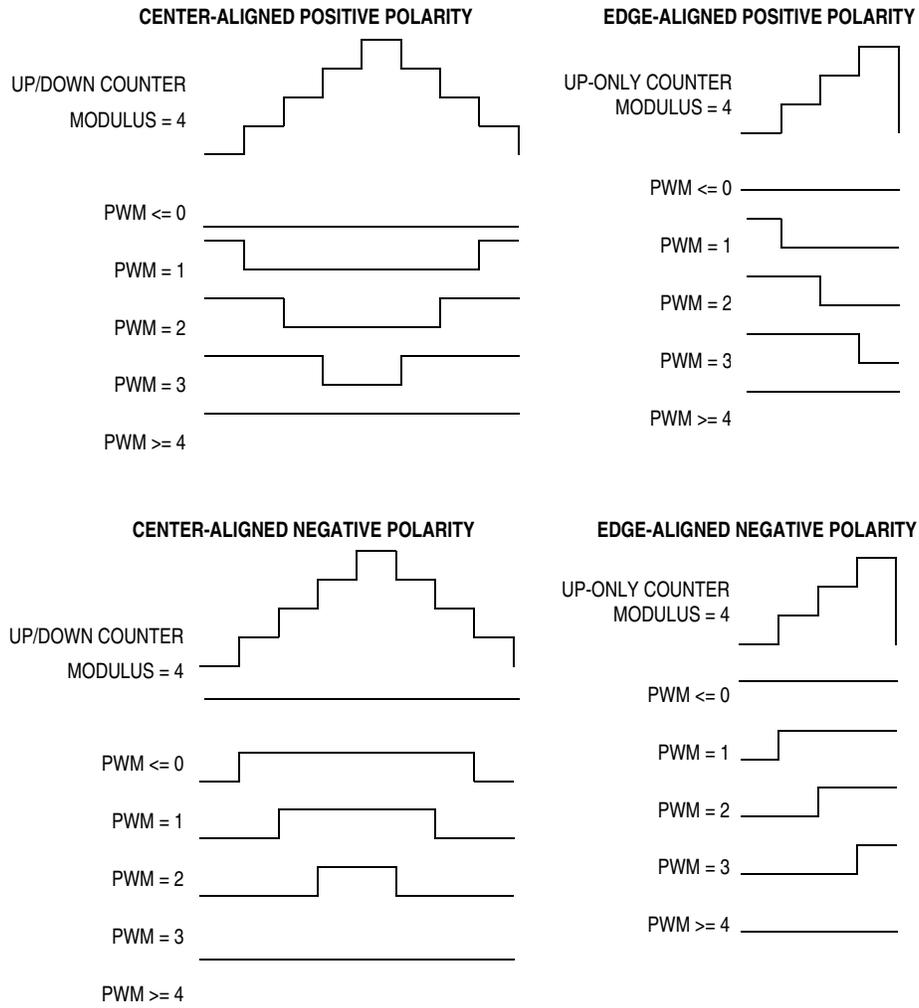
**Figure 12-21. PWM Polarity**
