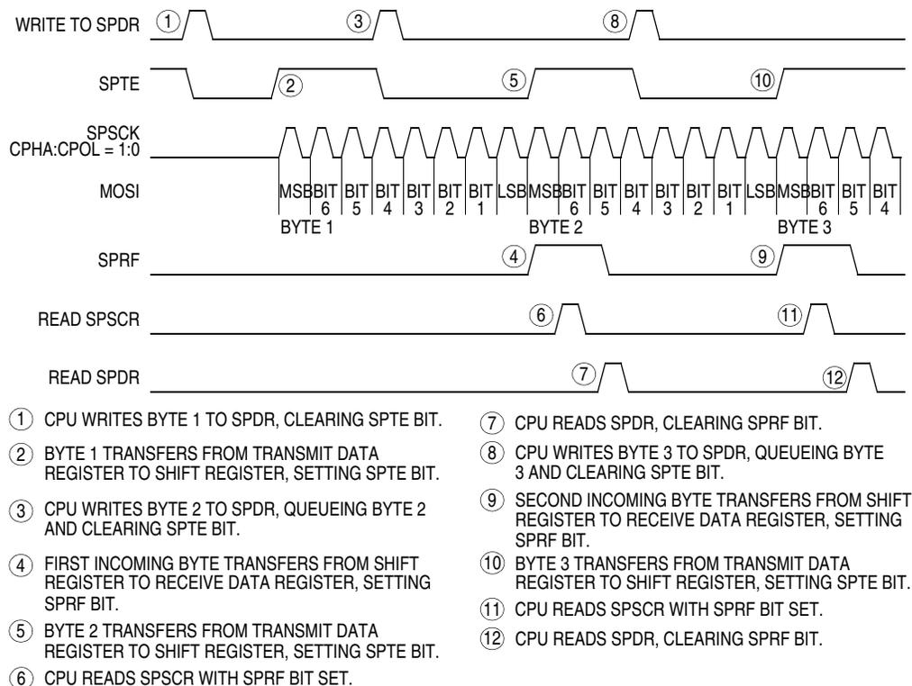
**Figure 15-12. SPRF/SPTE CPU Interrupt Timing**
