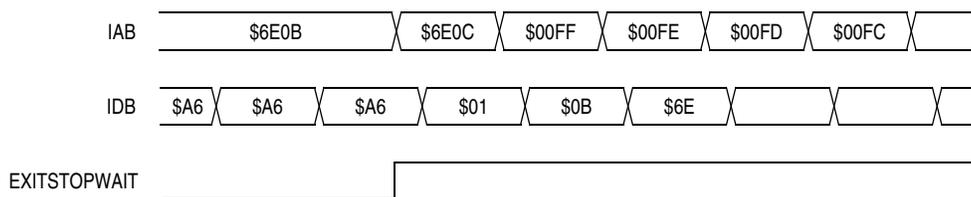
Note: EXITSTOPWAIT =  $\overline{\text{RST}}$  pin OR CPU interrupt
