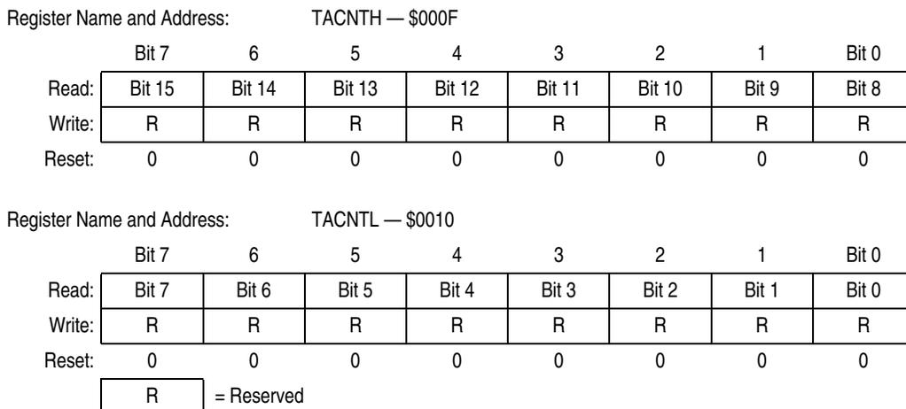
**Figure 16-6. TIMA Counter Registers (TACNTH and TACNTL)**
