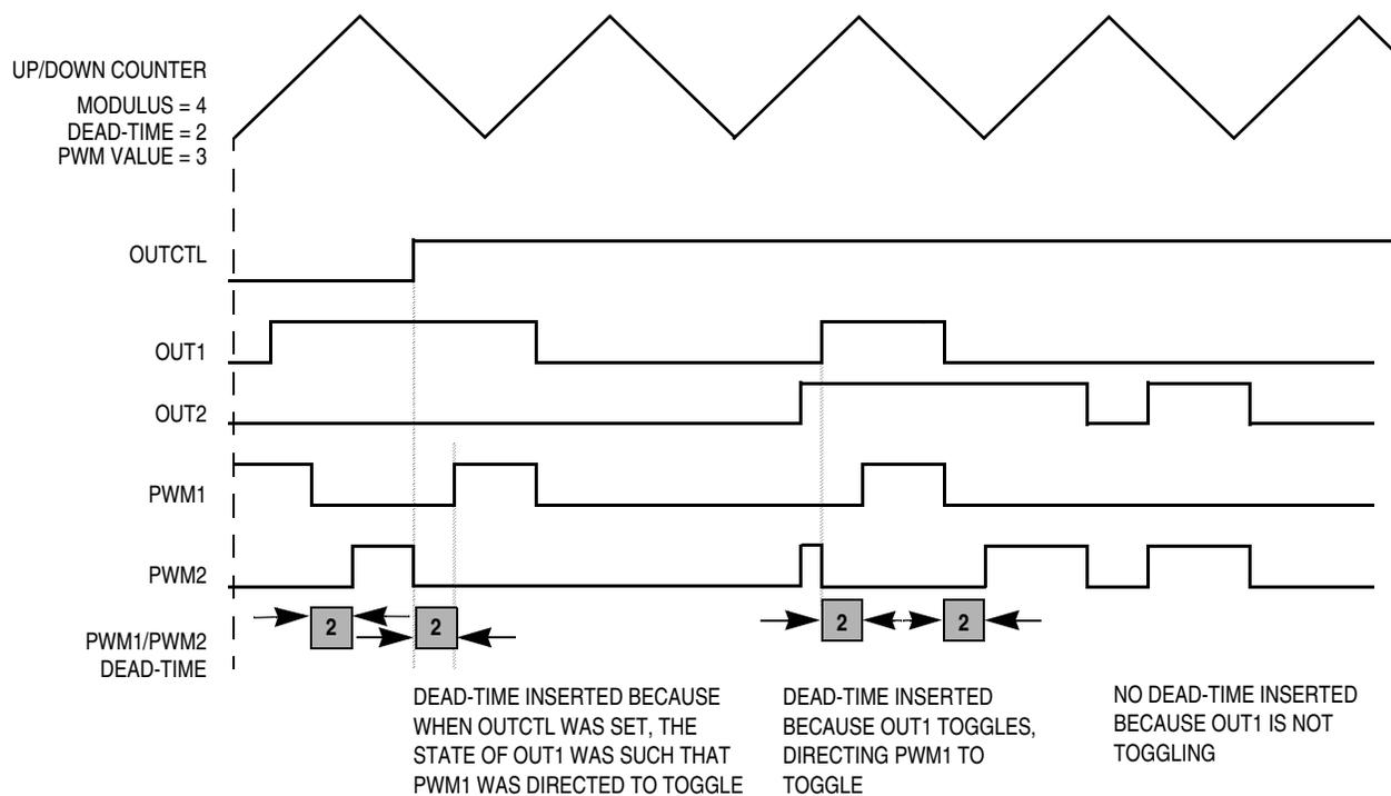
**Figure 12-24. Dead-Time Insertion During OUTCTL = 1**
