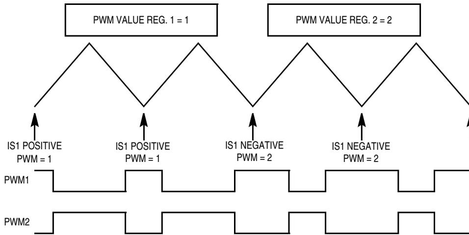
**Figure 12-20. Top/Bottom Correction for PWMs 1 and 2**
