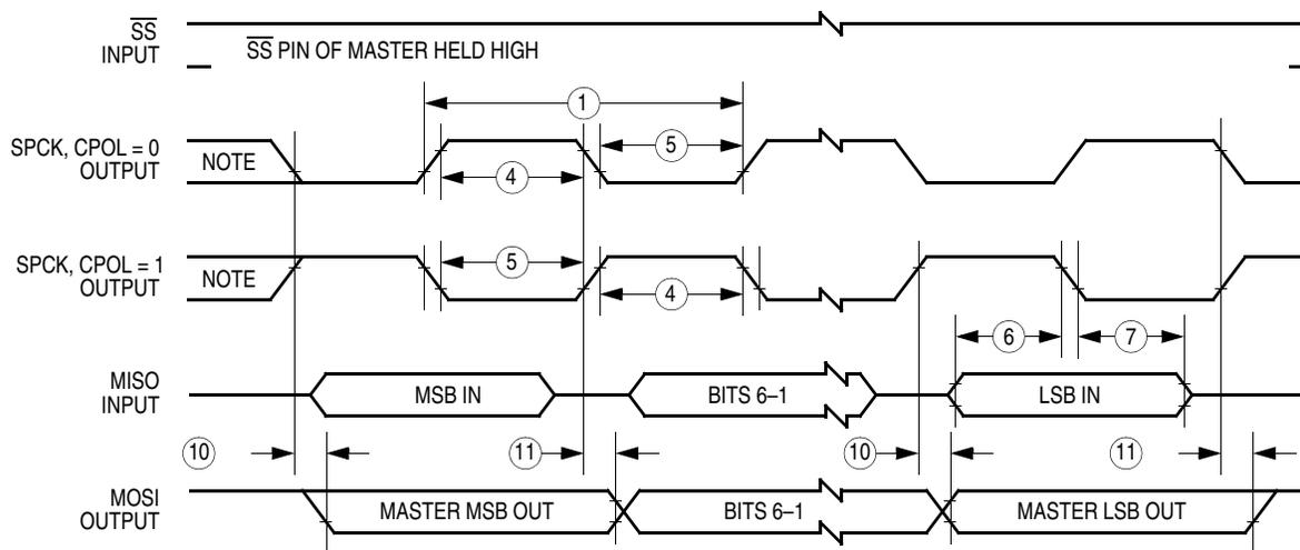
Note: This first clock edge is generated internally, but is not seen at the SCK pin.
