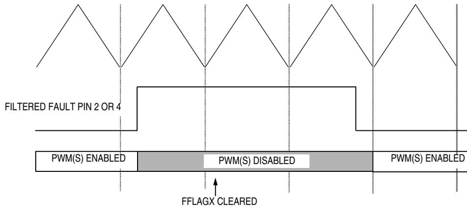
**Figure 12-30. PWM Disabling in Manual Mode (Example 2)**
