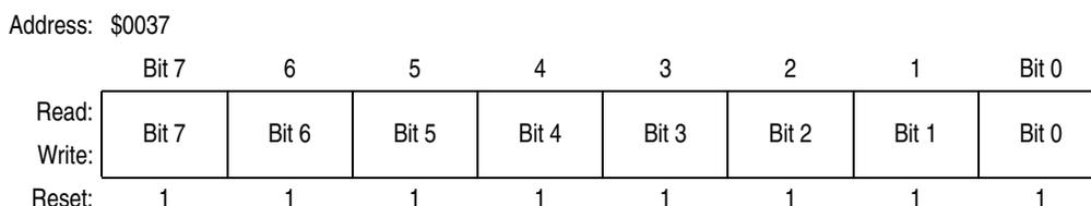
**Figure 12-25. PWM Disable Mapping Write-Once Register (DISMAP)**
