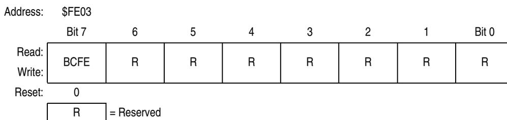
**Figure 18-7. SIM Break Flag Control Register (SBFCR)**
