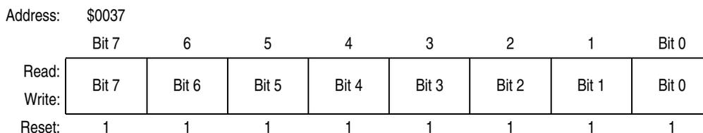
**Figure 12-42. PWM Disable Mapping Write-Once Register (DISMAP)**
