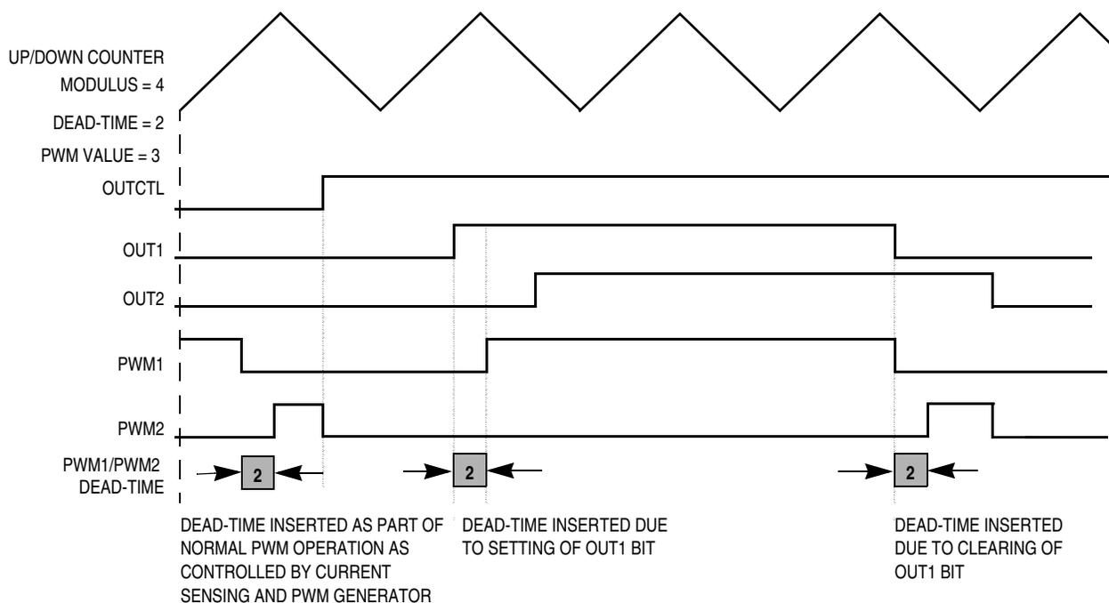
**Figure 12-23. Dead-Time Insertion During OUTCTL = 1**
