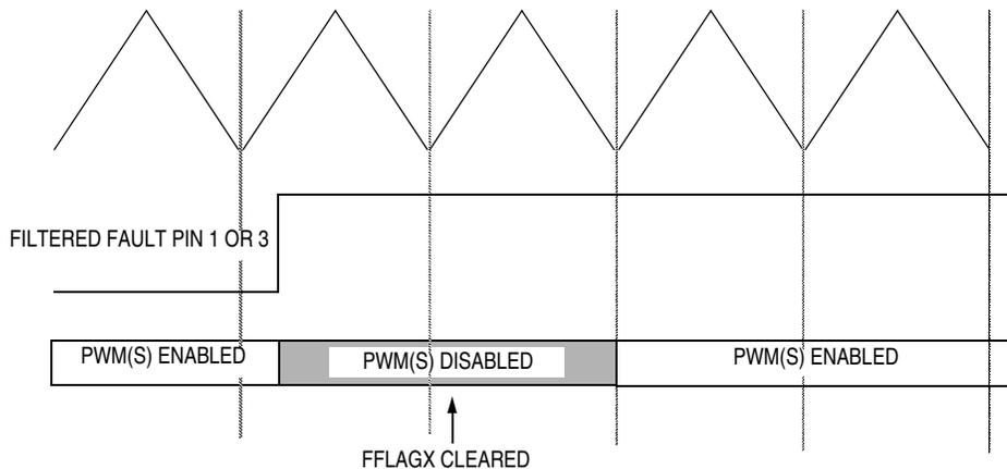
**Figure 12-29. PWM Disabling in Manual Mode (Example 1)**
