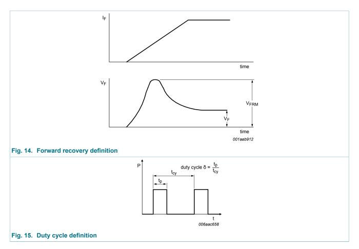
The current ratings for the typical waveforms are calculated according to the equations:  $I_{F(AV)} = I_M \times \delta$  with  $I_M$  defined as peak current,  $I_{RMS} = I_{F(AV)}$  at DC, and  $I_{RMS} = I_M \times \sqrt{\delta}$  with I<sub>RMS</sub> defined as RMS current.
