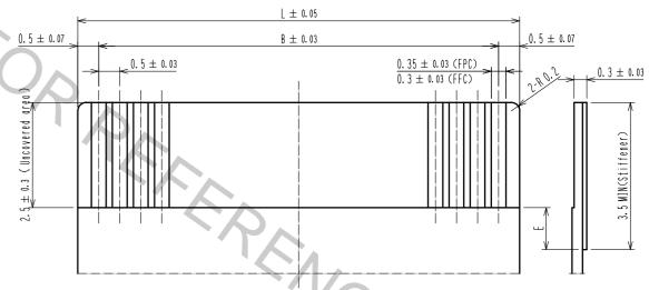
For FPC application, stiffener material is polyimid, heat cured adhesive. For FFC application, pay attention to the tolerance of FPC thickness at mating area. Dimension E must be 0.5mm minimum when the stiffener is shorter than 3.5mm.
