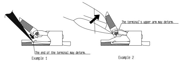
2. When operating the actuator, do not apply a force in the direction of the connector. The actuator may get pushed into the connector, causing damage to the connector.
