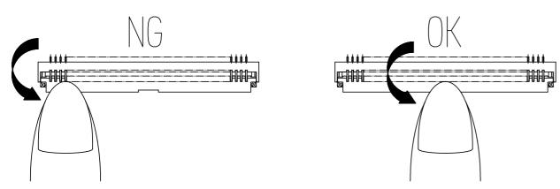
♦ Confirming the state of the lock Once it is locked, make sure that the actuator is parallel to the board. However, if the actuator approaches O degrees, make sure that it is not.
