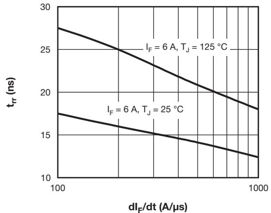
Fig. 7 - Typical Reverse Recovery Time vs.  $dI_F/dt$
