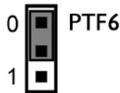
Puts the 3-axis accelerometer into sleep mode. The user may control PTF6 in firmware to enable or disable the accelerometer.
