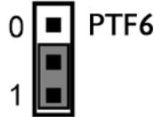
Enables the 3-axis accelerometer. This is the default setting.
