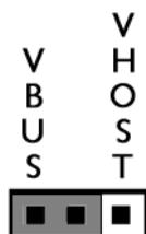
A jumper across 1 & 2 indicates that the Mini-USB will be powered from the bus. This is the default setting.
