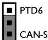
**Figure 8-4: Can Operation Mode Selection (J6)**
