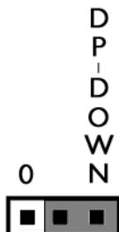
A jumper across 2 & 3 indicates that the USB\_DP\_DOWN signal controls the pull down of USBDP signal. This is the default setting.
