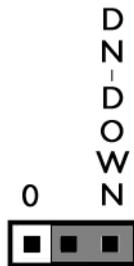
A jumper across 2 & 3 indicates that the USB\_DN\_DOWN signal controls the pull down of USBDN signal. This is the default setting.
