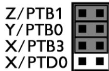
The accelerometer output signals are jumper-settable to PTB1, PTB0, PTB3, and PTD0. PTB3 and PTD0 share the same X-axis signal. By default, the X-axis signal is connected to PTB3.
